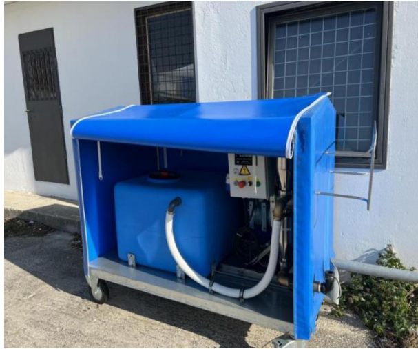
Mobile device for receiving and pumping fecal water from ships installed in marina Strožanac
