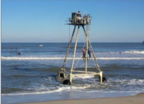
Figure 9: Coastal Research Amphibious Buggy (CRAB) used for beach profile measurements at the U.S. Army Corps of Engineers Field Research Facility, Duck, North Carolina. From Pranzini and Rossi, 2013)
