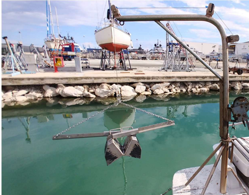
Figure 5. van Veen grab (0.1 m 2 ) for the sampling of macrofaunal communities
