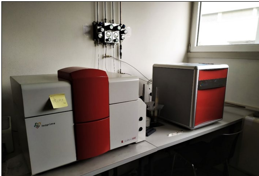
Figure 5: EA-IRMS instrumentation. On the right, there is the elementary analyzer "Elementar Vario Microcube"; on the left there is the "Isoprime100" mass spectrometer.
