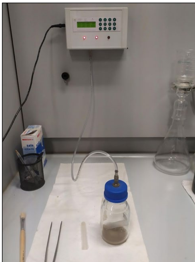
Figure 4: instrumentation used for calcimetric analyses.
