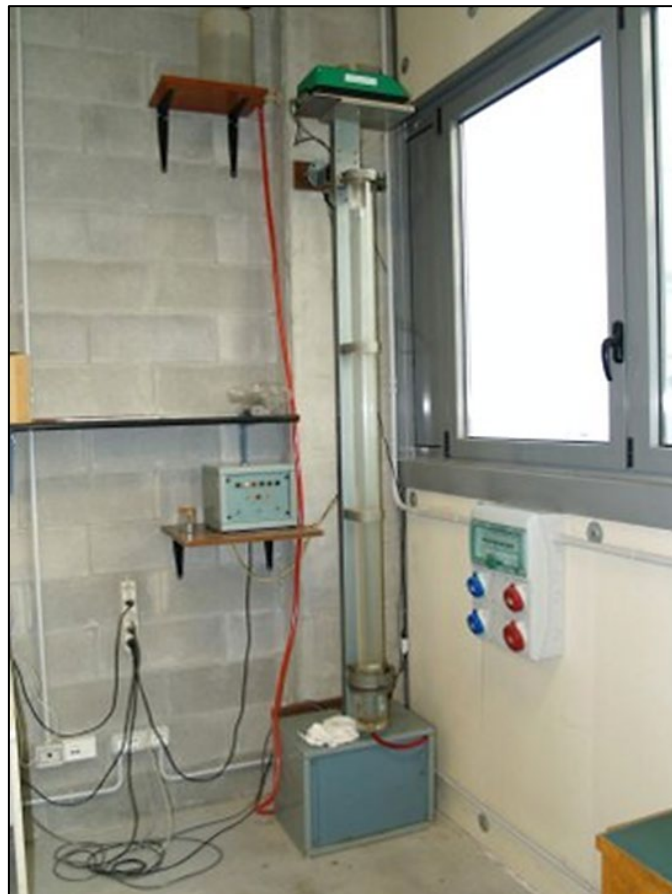
Figure 2: Sedimentation balance used for the analyses.
