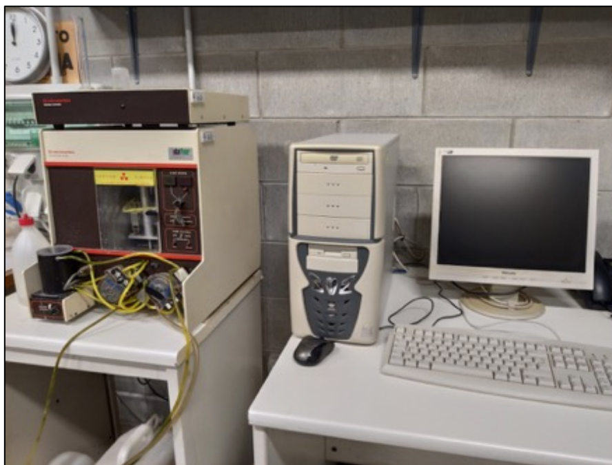
Figure 3: Instrumentation of the X-ray sedigraph used for the analyses.
