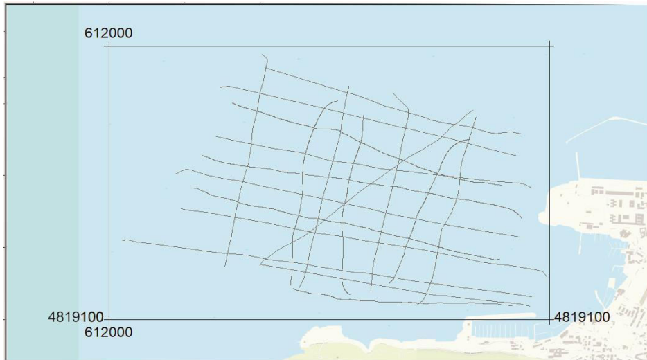
Figure 14. Position map of the boomer and sparker lines acquired in the Spinut area.
