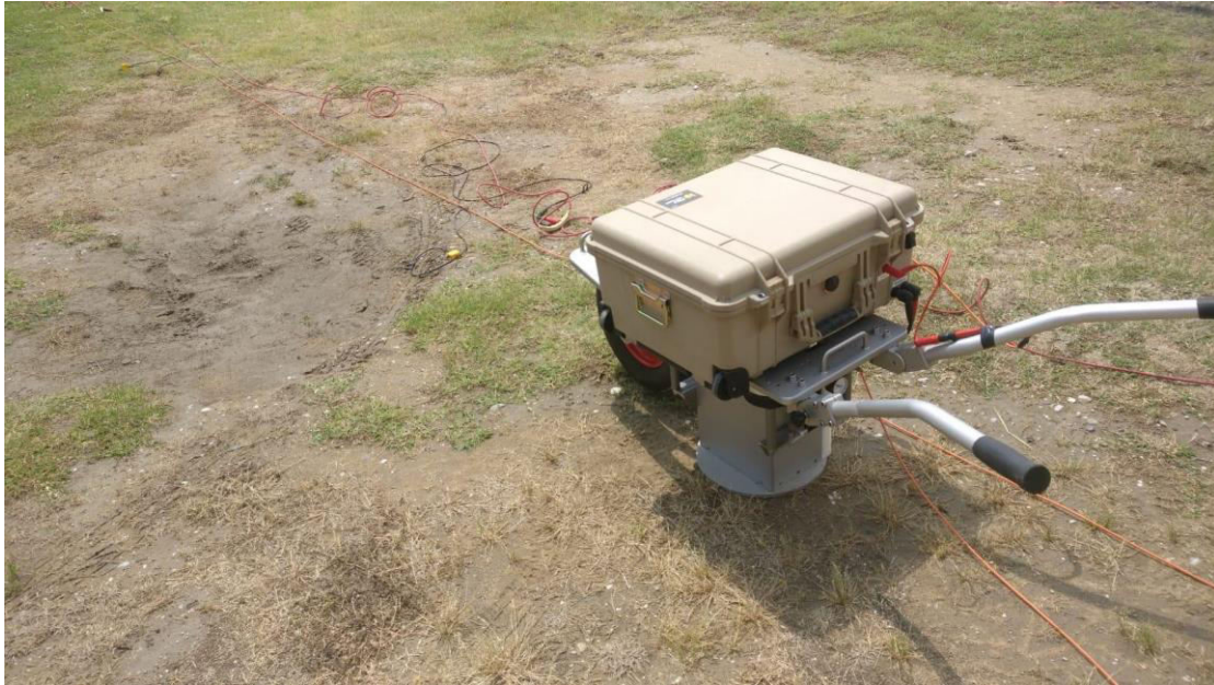
Figure 11. Vibroseis source Elvis VII from Geosym
