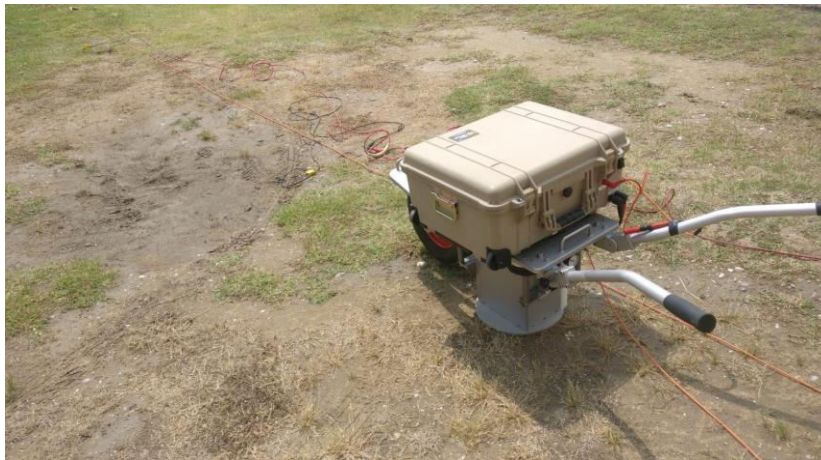
Figure 24. Vibroseis source Elvis VII from Geosym
