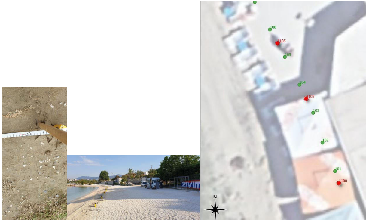
Figure 12. line set-up steps (a) deploy sensors and digitizers (b) coupling geophones to ground (c) detail of the map with stake numbers. The red symbols indicate the VP, the green dots the receiver's stakes
