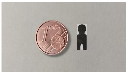
Figure 1. Photo of the phosphate sensor developed based on miniaturized plastic electrode showing its actual dimensions compared to a one-cent coin.
