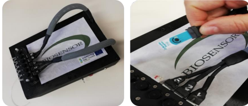
Figure 1. Dual electro-optical transducer prototype for the measurement of the chlorophyll a fluorescence and for the measurement of the current signals of algae under light illumination.
