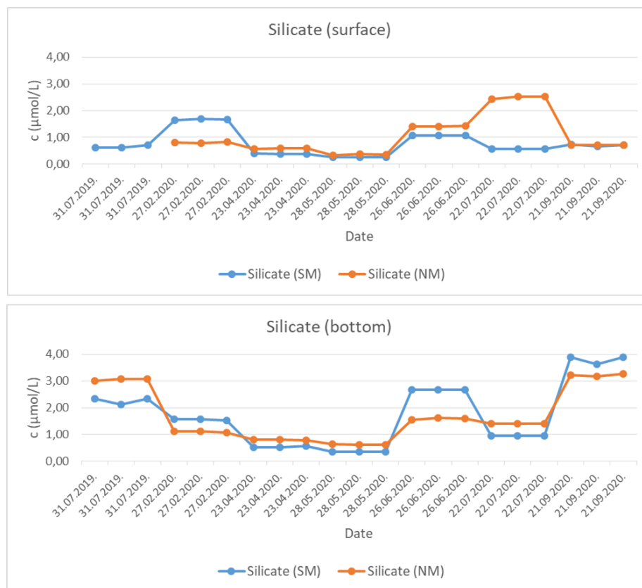
Figure 16. Comparison of silicate concentrations determined with standard method (SM) and new analytical method (NM) applied, shown as silicate monthly distribution in KB-SEA site samples investigated during 2019/2020. (Samples were taken in triplicates per each sampling date)
