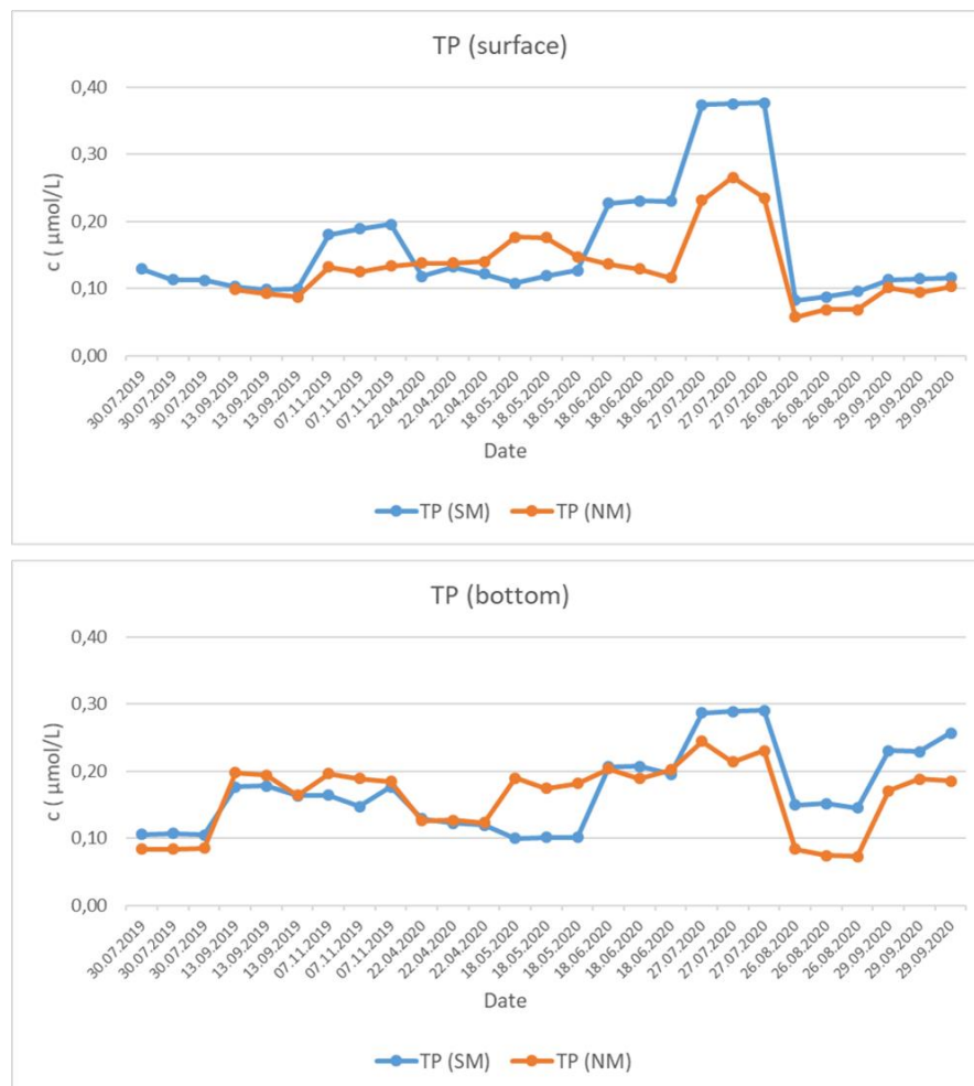
Figure 9. Comparison of TP concentrations determined with standard method (SM) and new analytical method (NM), shown as TP monthly distribution in ZD-SEA site samples investigated during 2019/2020. (Samples were taken in triplicates per each sampling date.)
