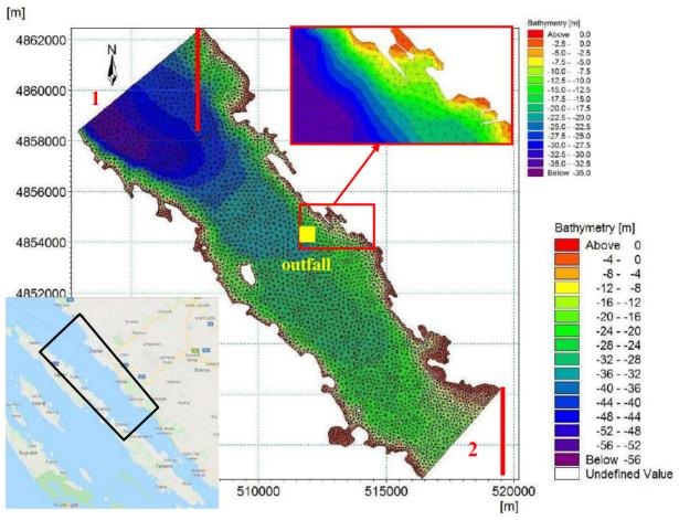
Figure 3 Numerical model spatial domain and respective discretization with finite volumes on bathymetry background (Mike 3fm, open boundaries are indicated with numbers 1 and 2)
