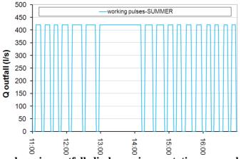
Figure 2 Zadar-centar submarine outfall discharge in nonstationary working mode (pulses) for sequence of characteristic "summer" day
