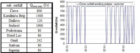
Figure 2 Main working characteristics of analyse submarine outfalls (left) and outfall discharge in nonstationary working mode (pulses) for sequence of characteristic "summer" day for Čiovo outfall (right)
