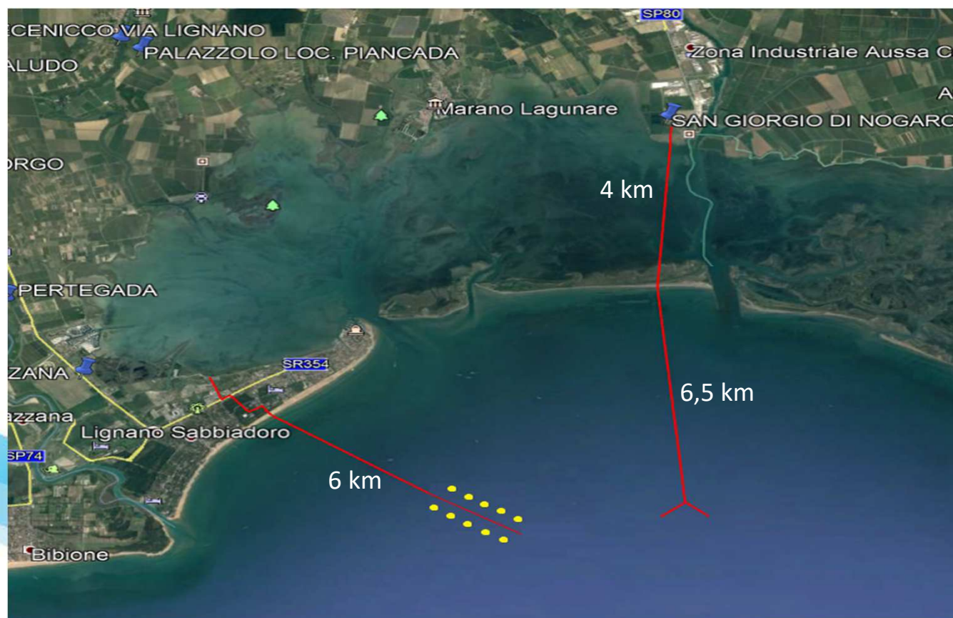
San Giorgio Di Nogaro – Underwater outfall pipeline layout
