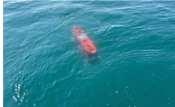
Figure 2 a) Underwater trajectory tracking with USBL. b) Blucy during USBL calibrations
