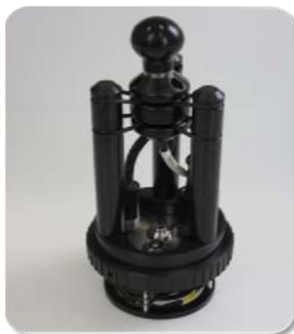
Figure 8 Hydrophone elastically attached to the casing avoiding case resonances
