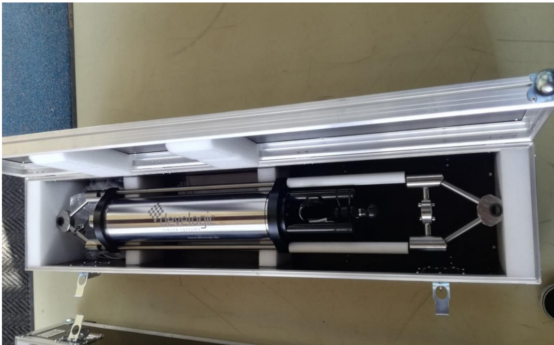
Figure 3-2 Autonomous passive underwater acoustic recorder Sono.Vault
