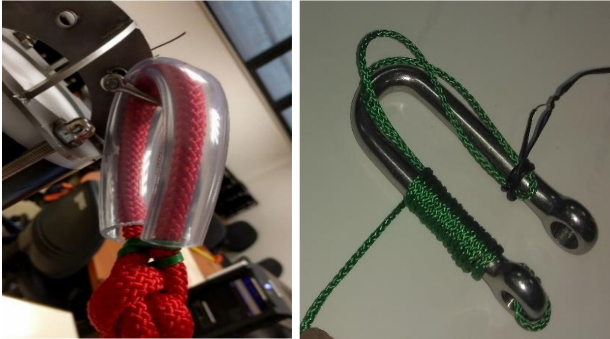
Figure 4 Examples for reducing unwanted sound from the deployment gear
