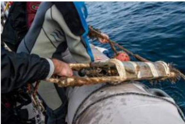
The hydrophone of Interreg-Soundscape project, managed by NGO "Cetacea Foundation", is recovered by the scuba team "Gianneri", Rimini (Italy). The hydrophone records continuously the sounds in the sea, for about three months. Every three months, it is recovered, cleaned of encrustations and the data are downloaded. Once memory cards are cleared, it is re-assembled and re-placed at sea for the next sampling period. Rimini, 10 October 2020. Photo courtesy of Elisabetta Zavoli.
