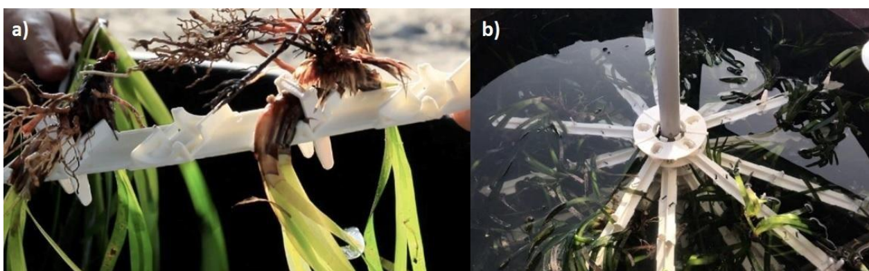
Figure 15. Ground fixing of cuttings to the arms (a), temporary storage of anchoring modules with cuttings/rhizomes.
