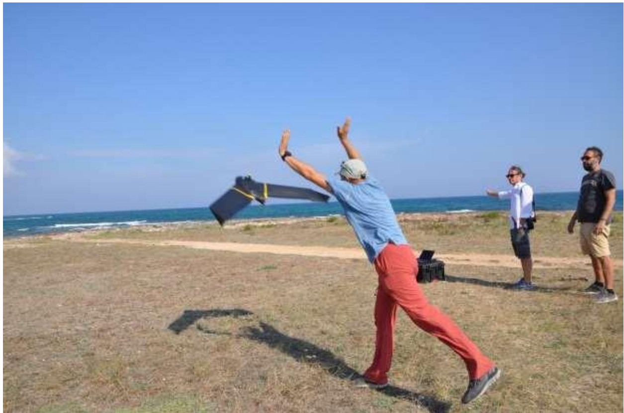
Fig.12: Torre S. Sabina, Carovigno (Br). Photogrammetric survey performed using UAS at Torre Santa Sabina (ph. UniSalento-F. Zongolo)
