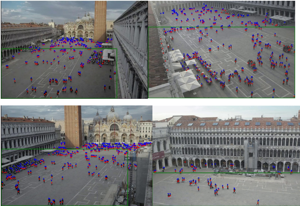
Fig. 2: examples of frames from the video cameras installed in San Marco square: the red box are the selected areas of the square to optimize the algorithms efficiency and to infer the presences in the whole square through a scaling of the density. The blue spots denote all the individuals (ground truth) whereas the red dots are the individuals detected by the the neural network.
