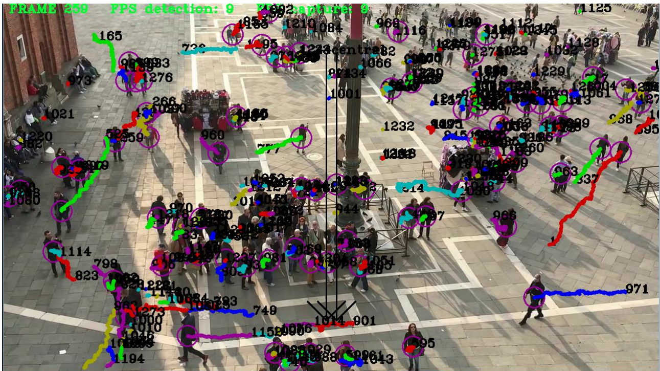
Figure 4.2: Example of crowd counting in San Marco Square in Venice: the number is an id associated to each detected individual and the curves denote the reconstructed trajectories from the video analysis.
