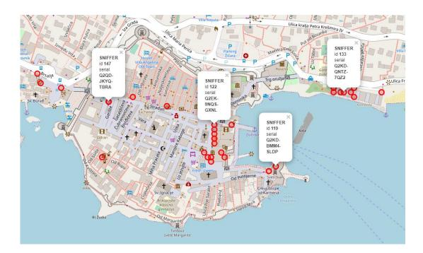
Figure 4: The red circles show the location of the Wi-Fi access points able to detect the presence of mobile device Wi-Fi connected in the Dubrovnik historical centre to perform the experimental campaign
