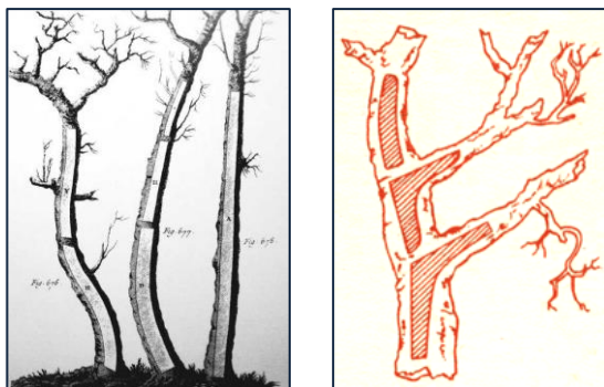
Identification of naturally curved timbers ( stortami ) in the trees, to be used in shipbuilding
