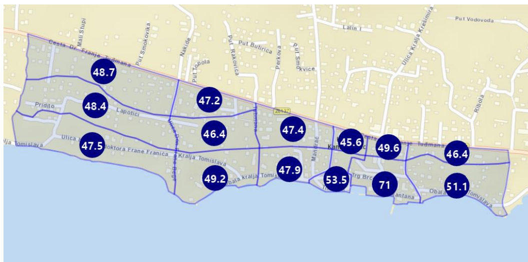
Figure 5. Results of combined risk analysis for seismic and flood hazard for Level 2 (Scenario S-F L2)
