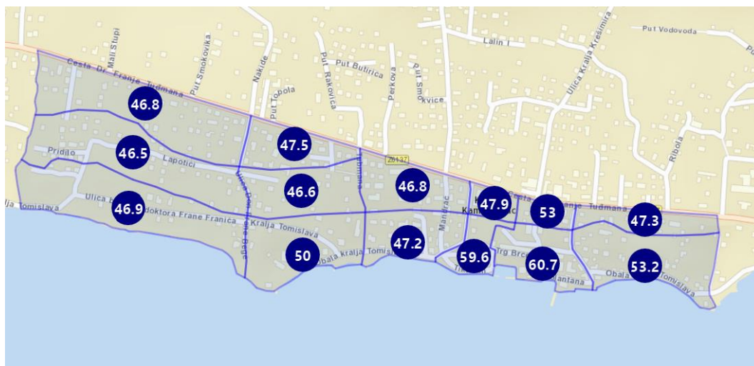
Figure 10. Results of combined risk analysis for seismic and flood hazard for Level 1 (Scenario S-F-EW L1)
