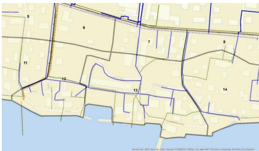
Figure 17. Overview of the water supply and drainage system separated by the boundaries of a homogeneous zone
