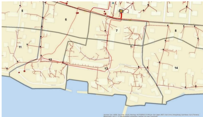
Figure 16. Overview of the power supply system separated by the boundaries of a homogeneous zone
