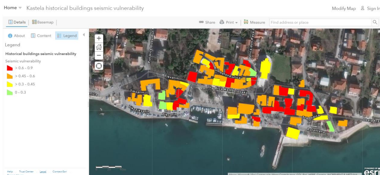
Fig. 4. Vulnerability classes of the buildings in historical core
