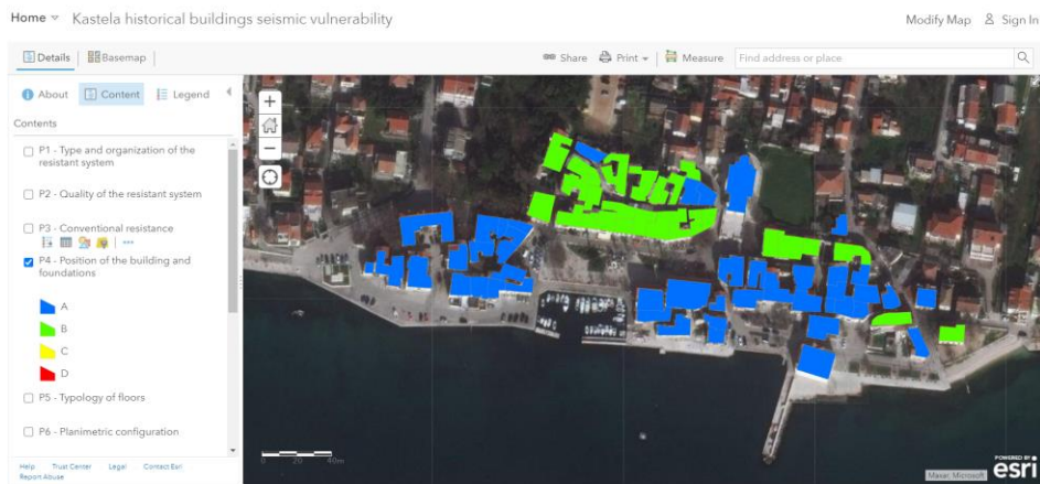
(d) Position of the building and foundation
