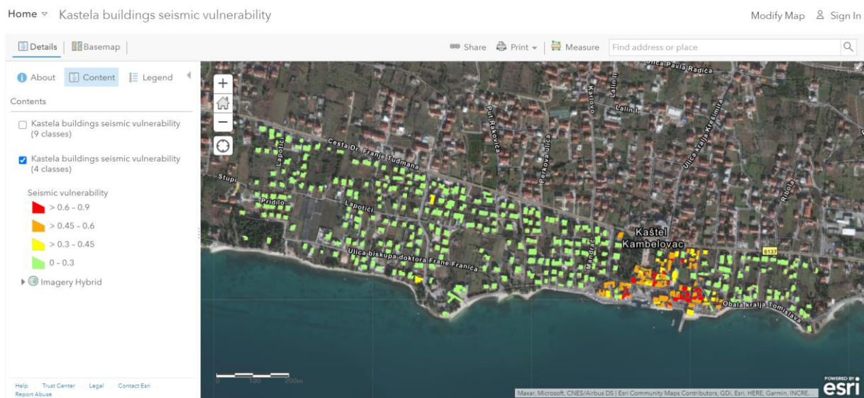
Fig. 29. Vulnerability of the buildings in the whole test site divided into 4 classes
