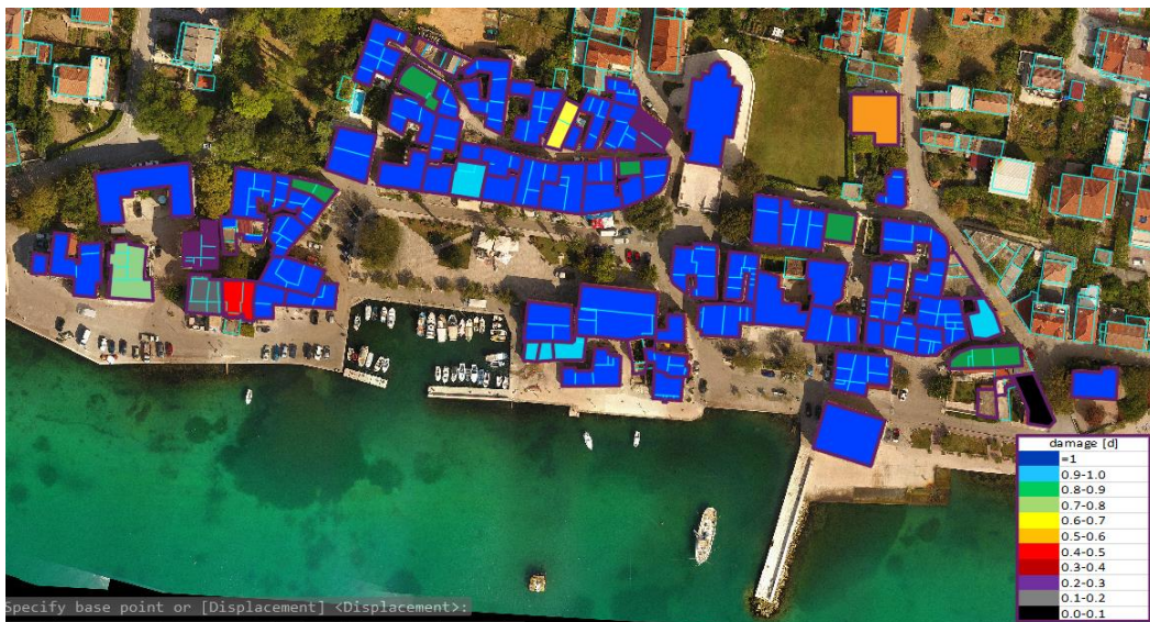
Fig. 49. Map of the damage index for PGA = 0.11 g and a return period T = 95 years
