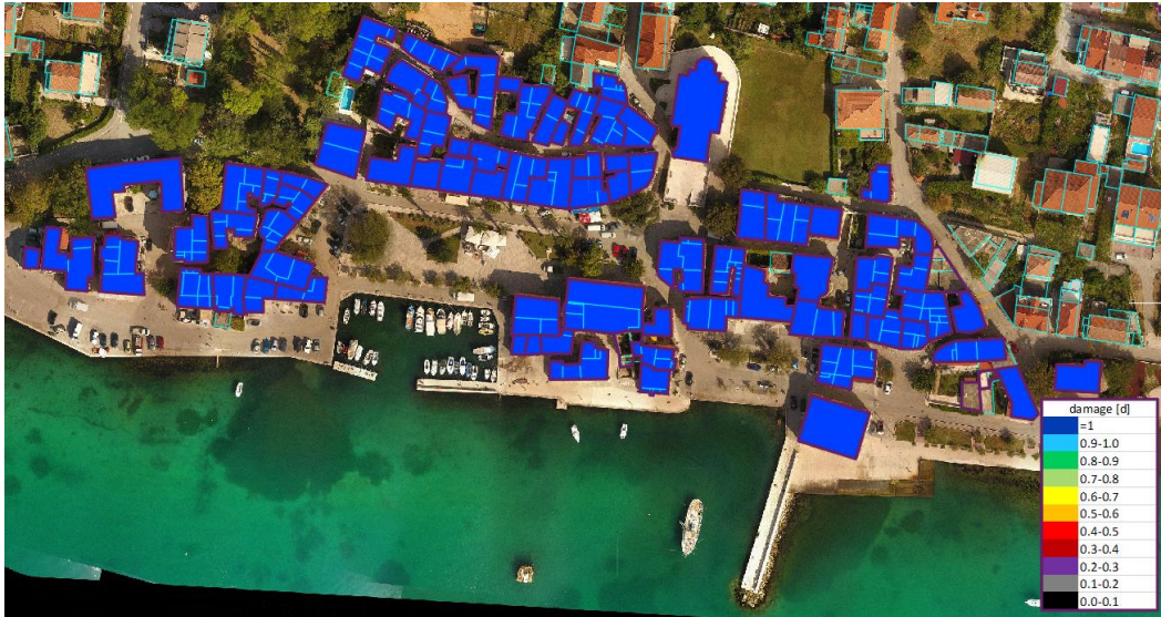
Fig. 50. Map of the damage index for PGA = 0.22 g and a return period T = 475 years
