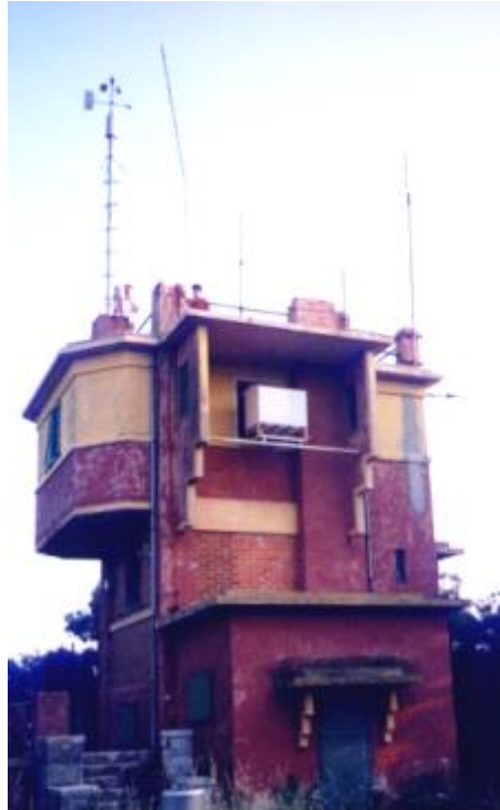
Figure 26. The position of the anemometer on the roof of meteorological station Split Marjan
