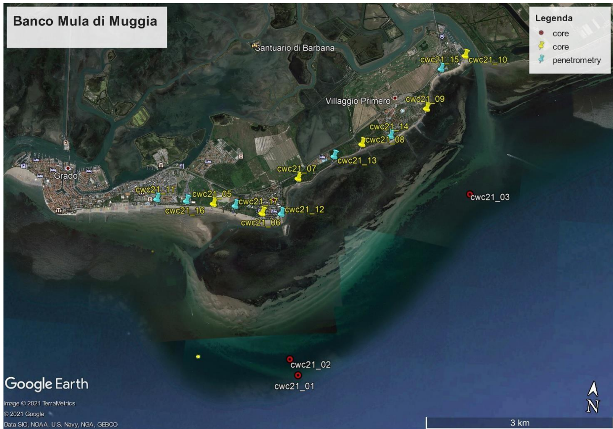
Figure 3: red and yellow dots represent cores; light blue dots represent penetrometries.
