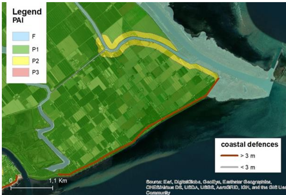
Figure 3-50 - Areas considered at different hydraulic hazard in the pilot site area (from PAIR)
