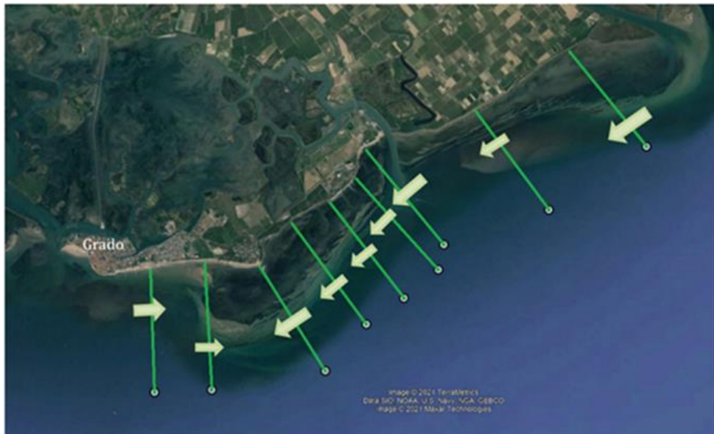
Figure 3-42 Representation of longshore transport for the entire area
