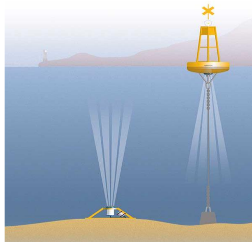
Figure 3.4.31. Example of acoustic Doppler current profiler (ADCP) configuration.
