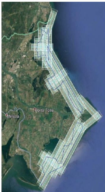
Figure 3-73: 2018 Lidar flight over the Po Delta area - from Veneto Region
