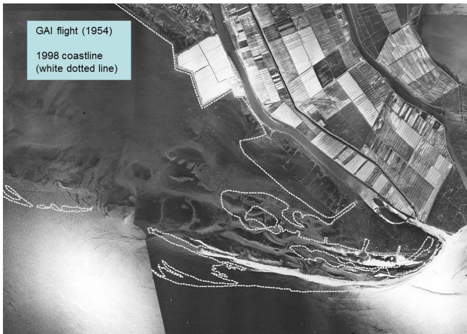
Figure 3-104: Comparison between aerial images (GAI flight, 1954 and IT2000 flight, 1998): river mouth is stable whereas spit shows new branches in distal portion and islands.
