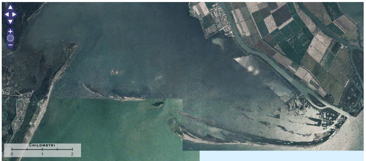
Figure 5-34: The spit is truncated by a new lagoonal inlet and a wide emerged sand bank is isolated between the reduced Scannone and the Volano spit.
