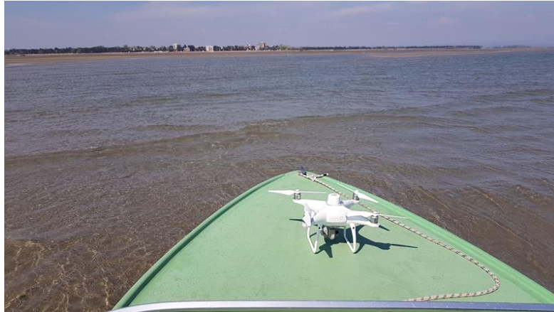
Figure 3-42: The APR (Remote Piloted Aircraft) DJI Phantom RTK used for the survey.
