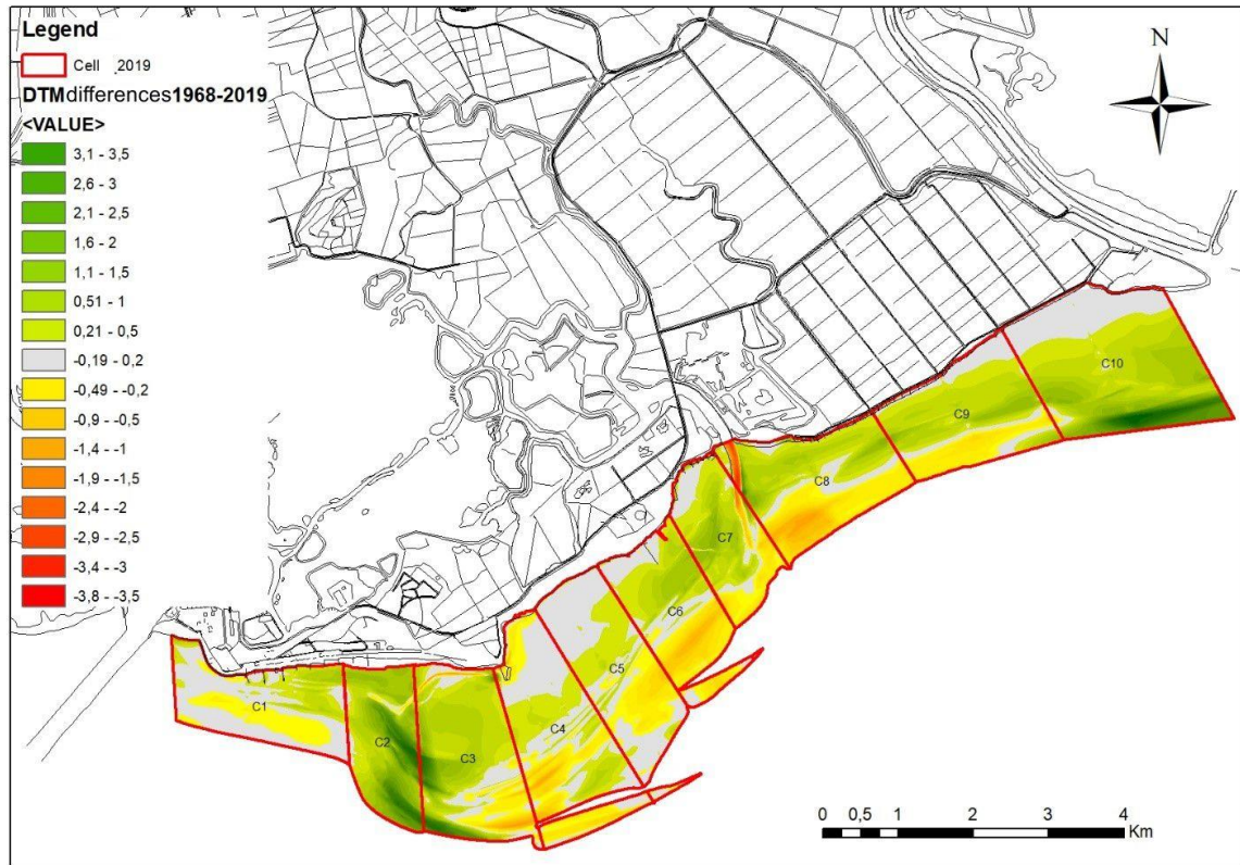
Figure 3-60: Map of altimetry differences from 1968 to 2019 with, superimposed, a geometric partition in littoral cells.
