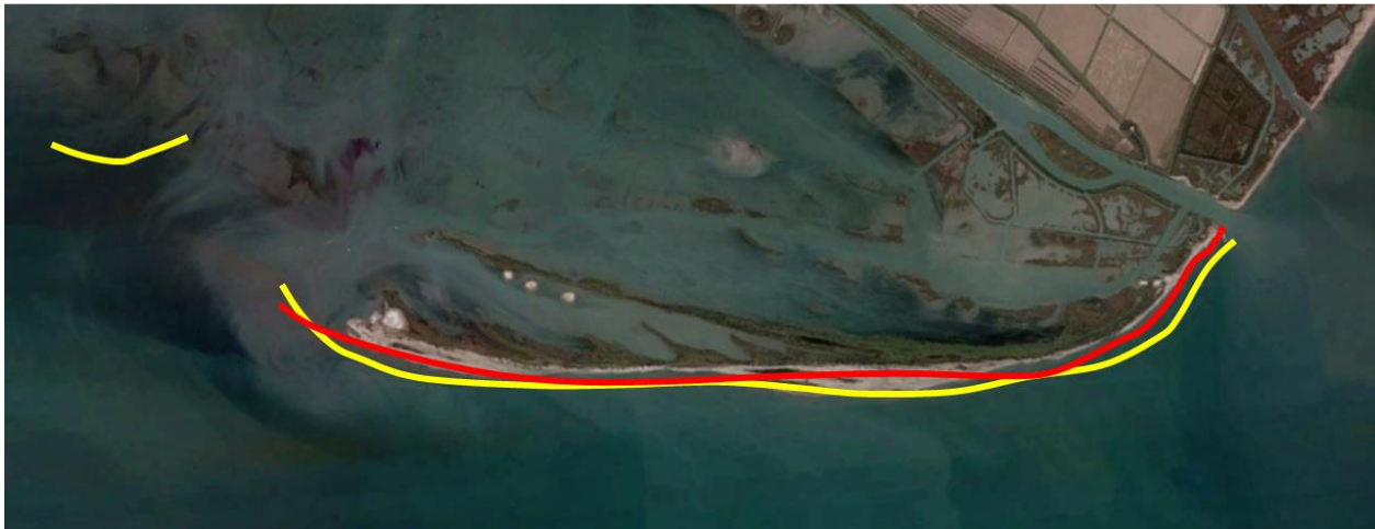
Figure 3-106: Comparison between satellite image of 2018 and 2003 coastline (yellow line) and 2013 coastline (red line): the figure shows the loss of the island in the west sector and regression in several points.
