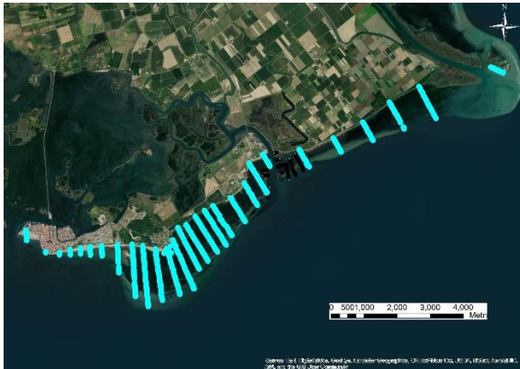
Figure 3-39: Topographic surveys during 2019, shoreline surveys
