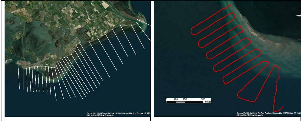
Figure 9-2 Survey pathways for bathymetric data: (left) geometrical approach and (right) additional surveys to detect bars not parallel to the general shoreline arrangement.
