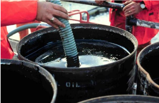
Picture 8: Filling an open top oil drum
