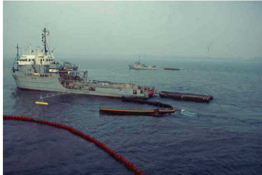
Figure 8: Skimming barrier with incorporated skimming device deployed from a single vessel
