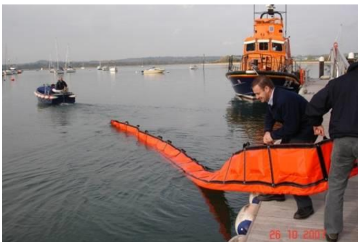
Figure 2: Fence boom being deployed from shore sea
