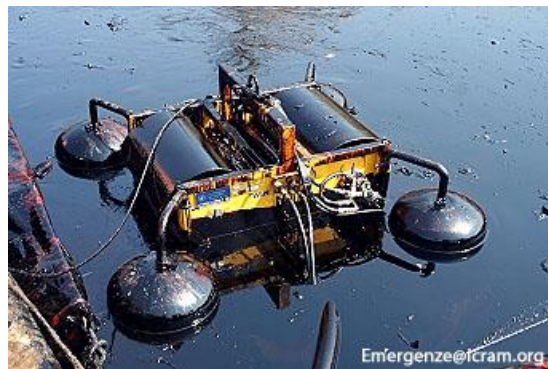
Figure 4: Operating principle and an example of an oleophilic drum skimmer
