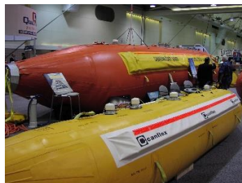
Picture 2: Towable floating (flexible) tank
