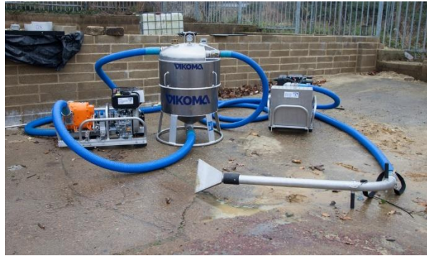
Figure 1: Operating principle and an example of a direct suction / vacuum skimmer
