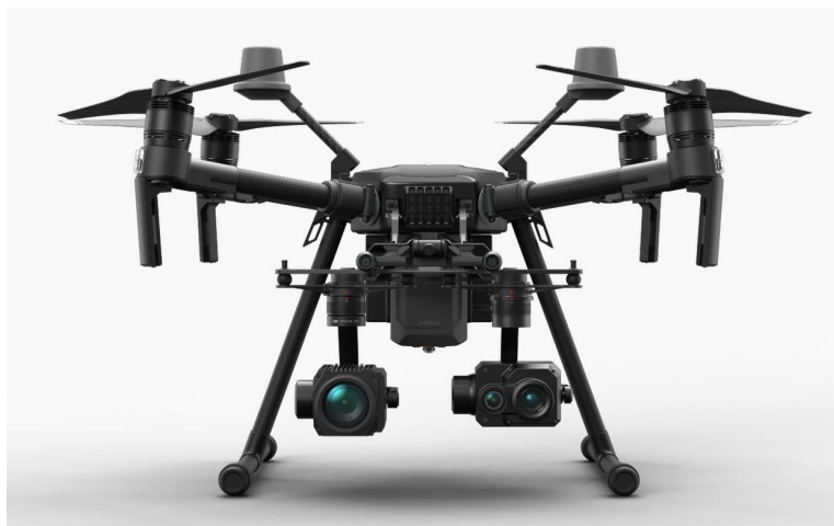
Figure 7. An example of a drone with an integrated RGB and thermal camera
