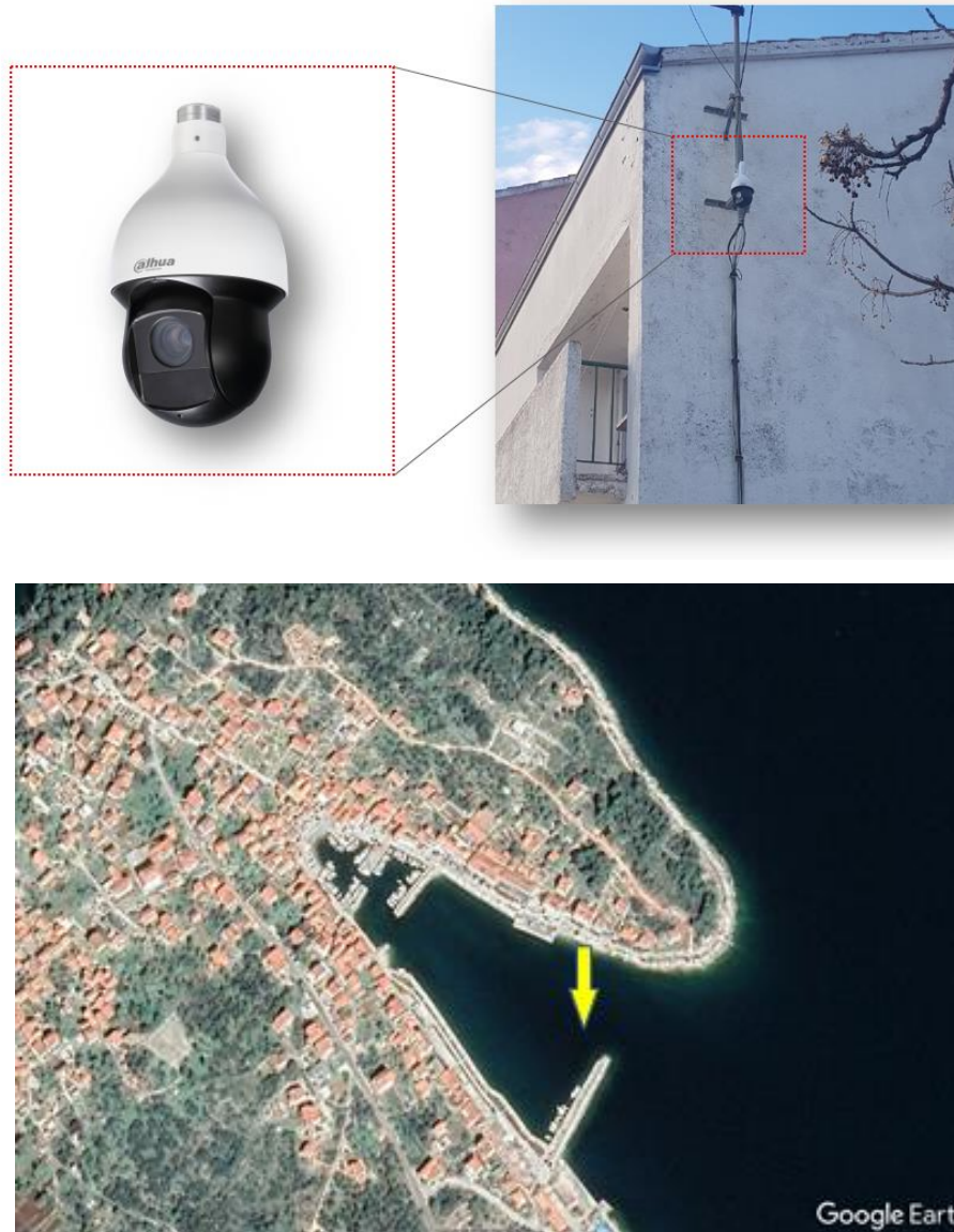
Figure I-9. Camera DAHUA SD-59230U-HNI used for monitoring in the PEPSEA project mounted on the wall of the Harbor Master's Office, and the direction in which the camera is facing (yellow arrow)
