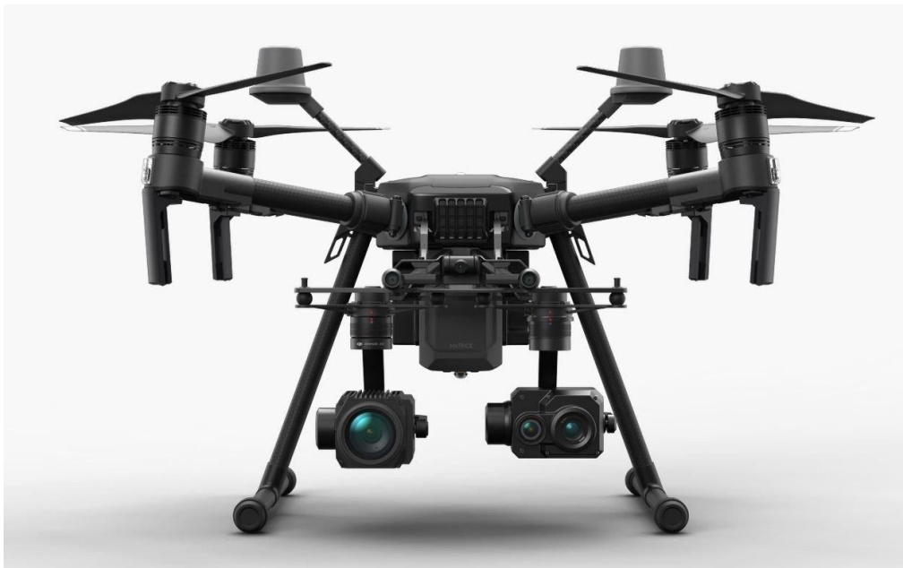
Figure I-11. An example of a drone with an integrated RGB and thermal camera
