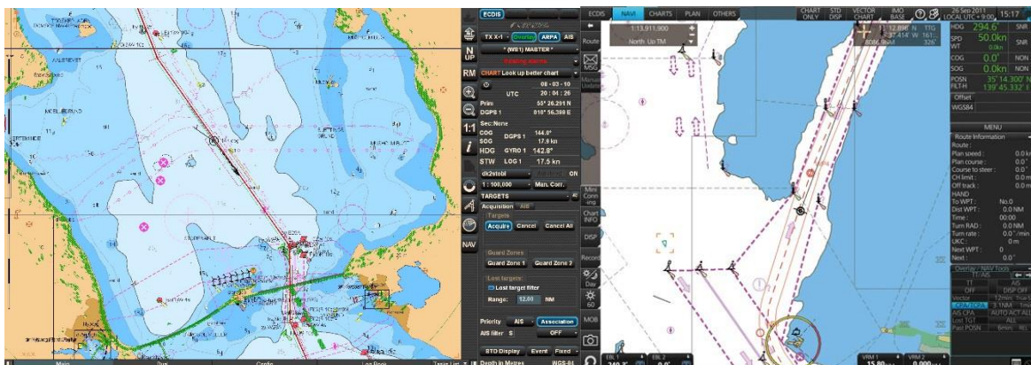
Figure I-5. Ship's electronic chart (ECDIS).
