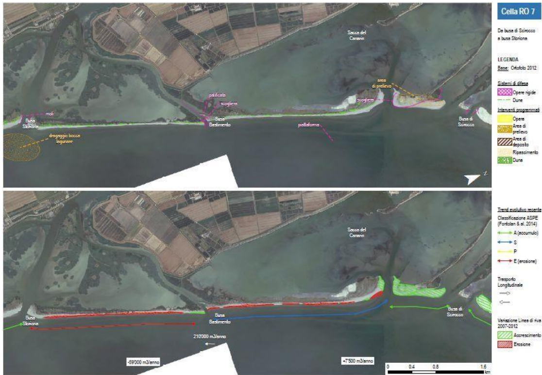
Figura 3-2 Defense strategy, interventions and solid transport trends in the Sacca del Canarin littoral. Source: Ruol e Pinato, 2016
