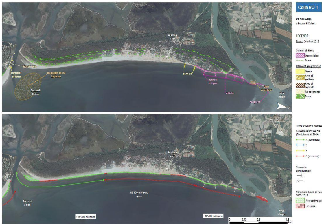
Figura 3-1 Defense strategy, interventions and solid transport trends in the Caleri littoral. Source: Ruol e Pinato, 2016.
