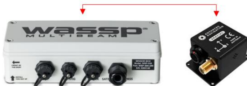
Slika I-15. WASSP Sensor Box s integriranim Advanced Navigation Spatial IMU WSP002-INU (prema: ENL Group, 2016; URL10)
