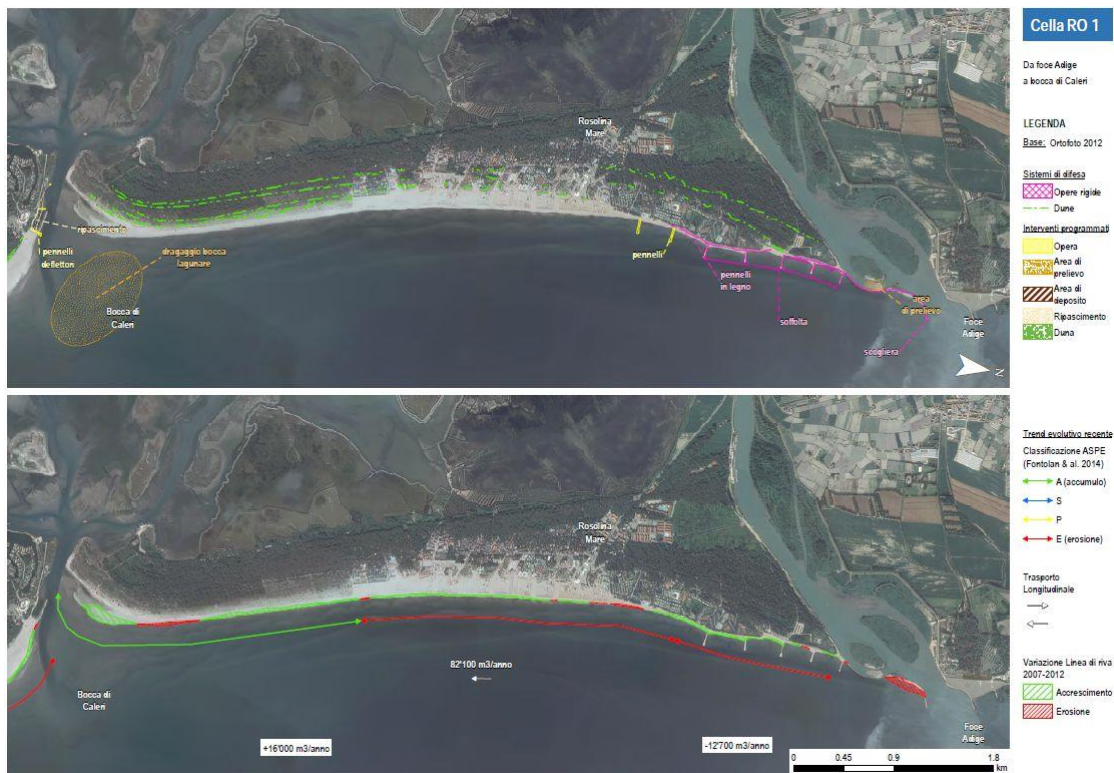
Figura 1-1 Defense strategy, interventions and solid transport trends in the Caleri littoral. Source: Ruol e Pinato, 2016.
