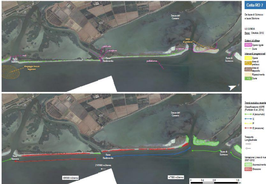
Figura 1-2 Defense strategy, interventions and solid transport trends in the Sacca del Canarin littoral. Source: Ruol e Pinato, 2016
