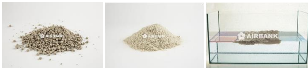
Figure 9: left, granulated OKO-PUR; middle powdered OKO-PUR; right OKO-PUR during an adsorption test from the water surface. (source : https://www.airbank.it/it/p/1/assorbente-legante-in-polvere-e-granuli-a-saturazione-totale ).
