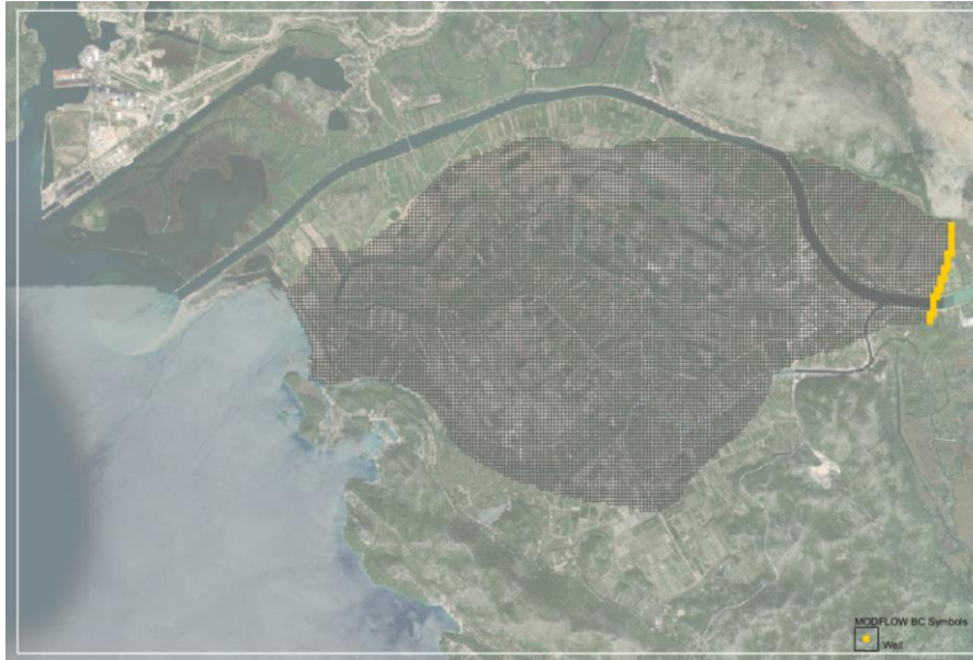
Figure 26 Specified flow in the layer of gravel
