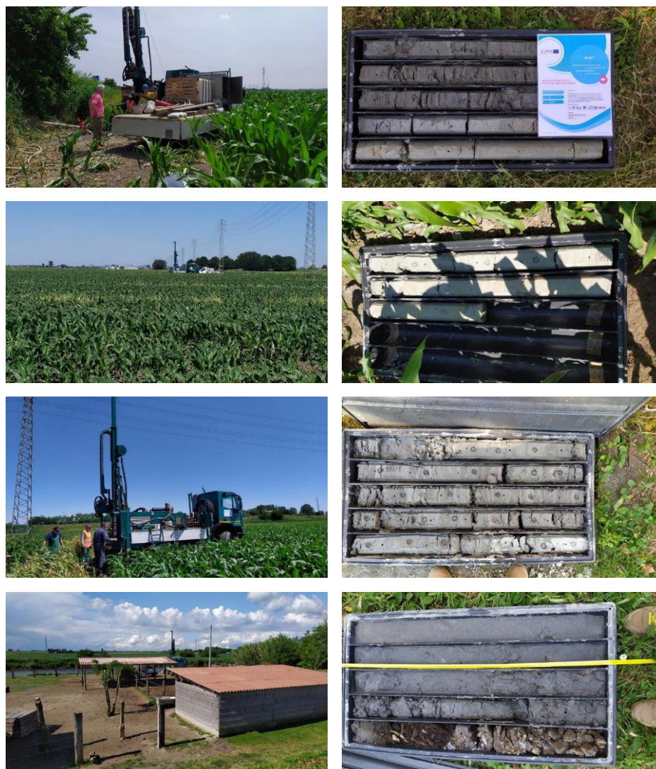
Fig. 3 – Example of drilling operation and core samples.
