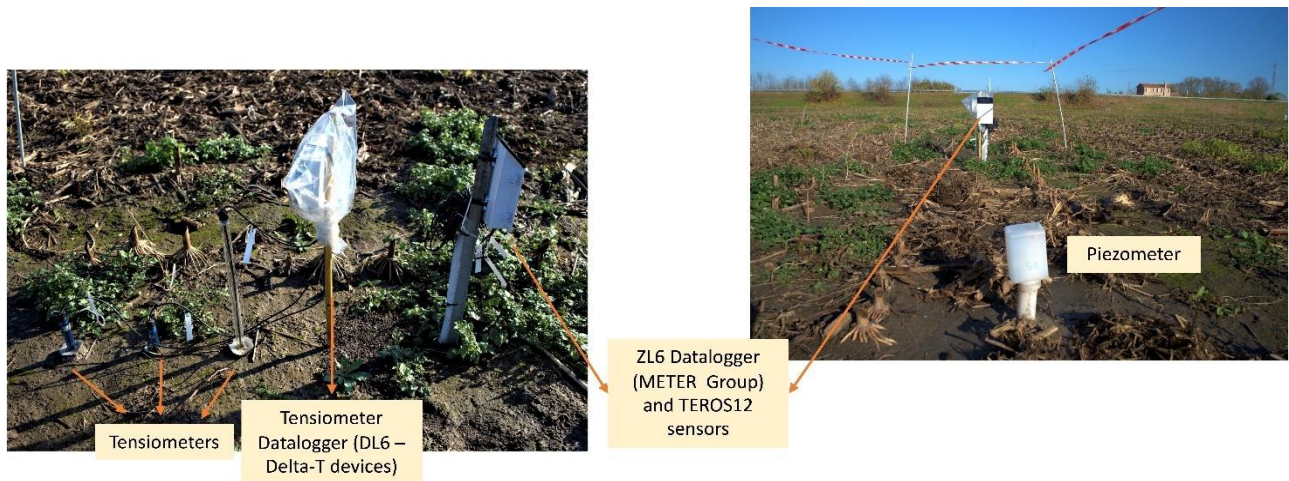
Fig. 31 Picture of the monitoring station with soil sensors, data loggers, and piezometers. The soil moisture, EC, and T sensors are not visible because they are completely into the soil.
