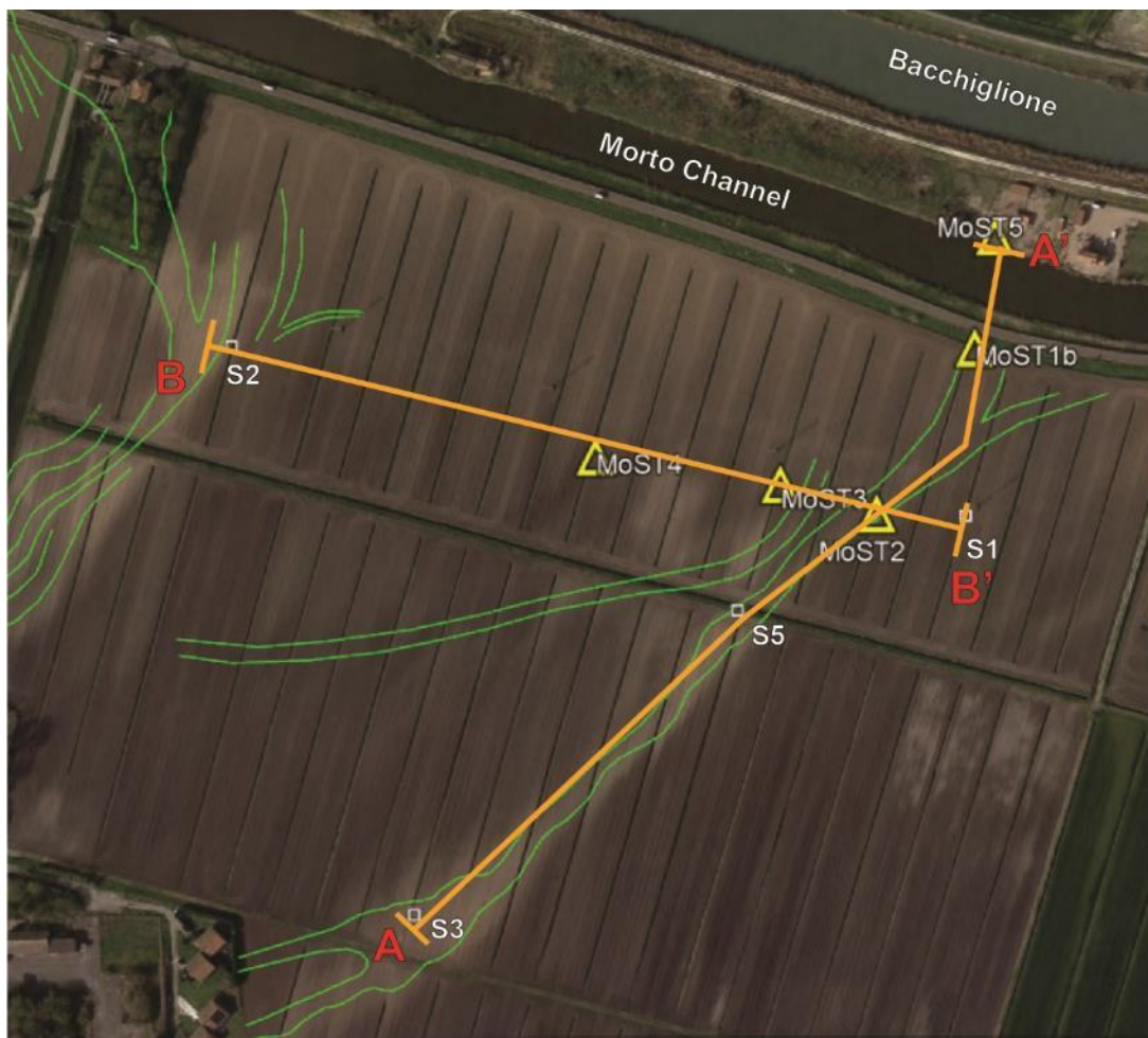
Fig. 15 – Map of the test site reporting the localization of the two stratigraphic sections (A-A', B-B'). The surficial sandy geomorphological bodies are indicated with green lines. The yellow triangles represent the MoST1-MoST5 wells, while the white squares the S1-S5 wells.
