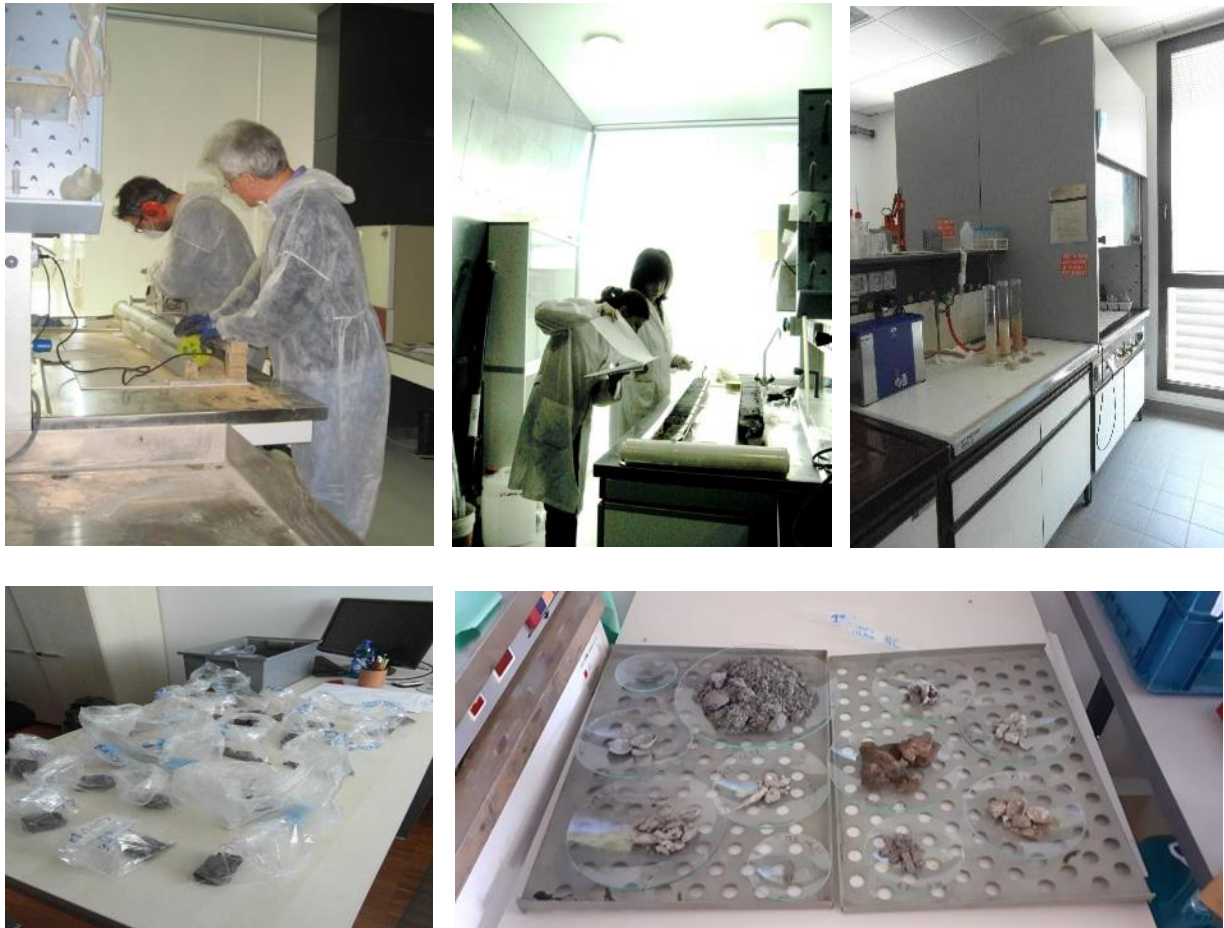
Fig. 5 – Activity at CNR lab: Core splitting, samples description and preparation for sedimentological analysis.
