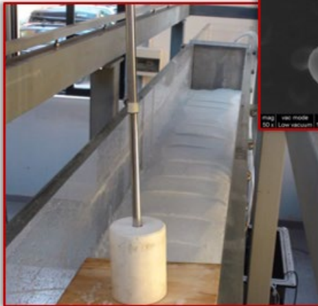
Sieving and compaction by impact (thickness of layers: 5 cm)
