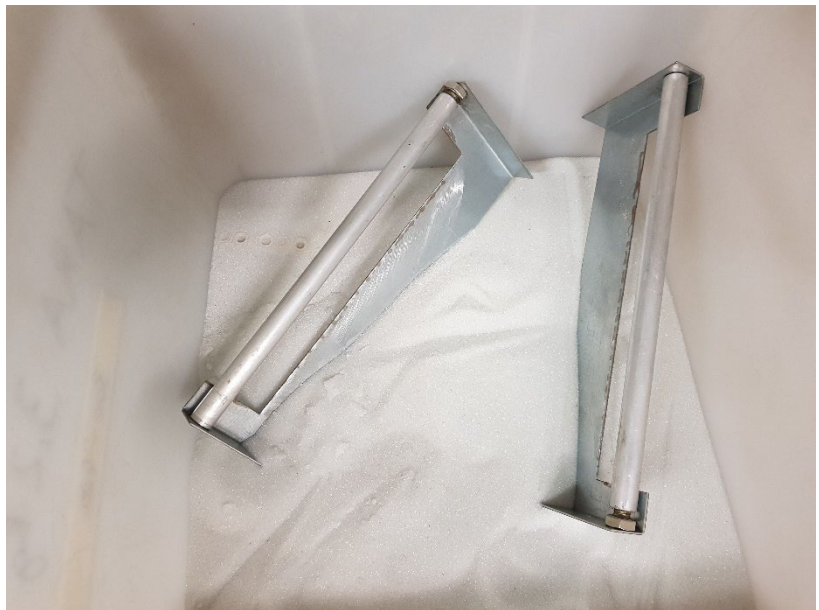
Figure 8 - Specially manufactured steel blades used to realize volumes at multiple distances of 20 cm in the same 5 cm thick layer
