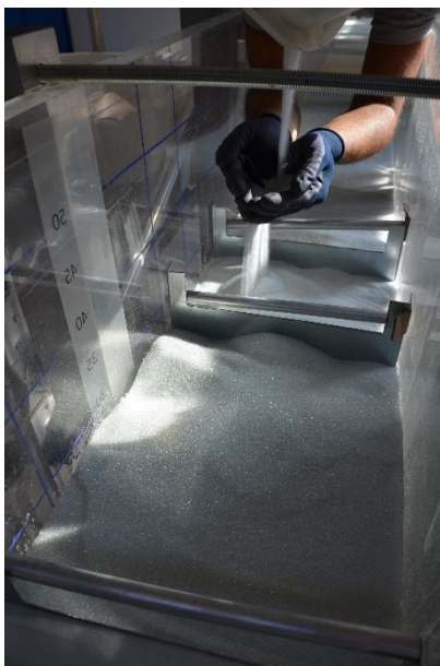
Figure 8 - Specially manufactured steel blades used to realize volumes at multiple distances of 20 cm in the same 5 cm thick layer
