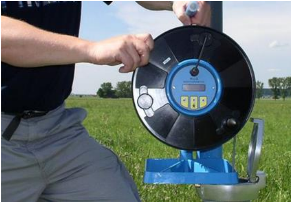
Figure 5 SEBA multi parameter gauge used for pro filing conductance at Neretva site
