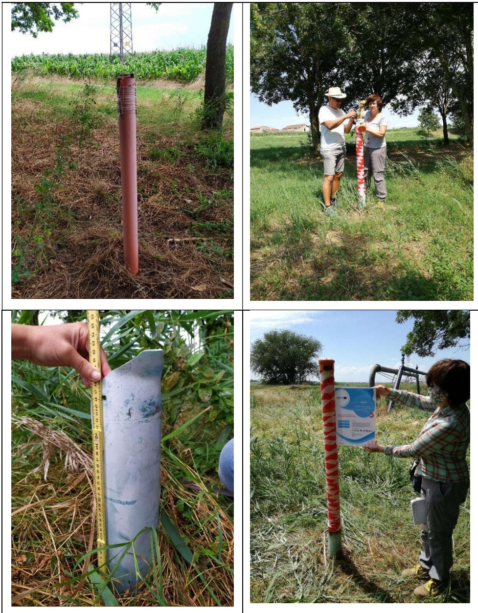
Fig. 5 – Examples of old piezometers used in the past, before and after restoration to be included in the MoST project.
