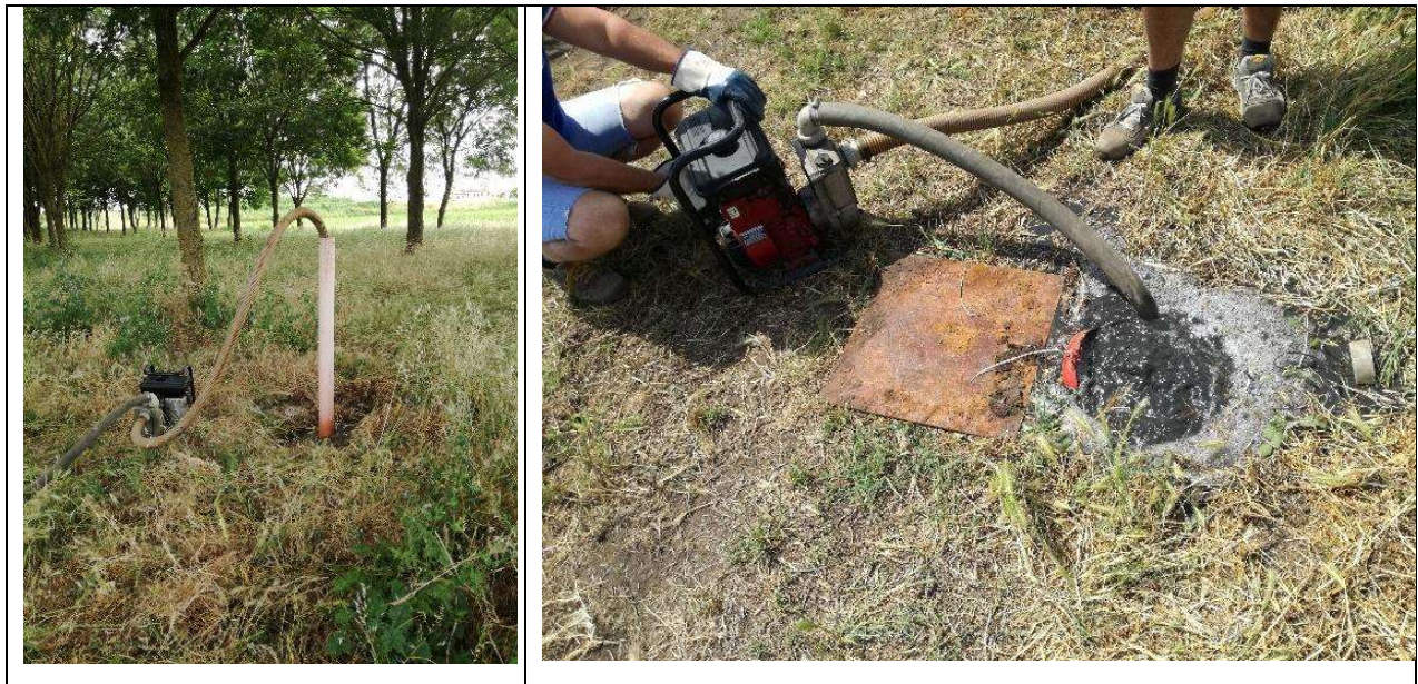
Fig. 6 – Examples of old piezometers cleaning.
