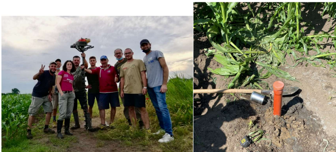
Fig. 35: Instrumentation used to establish the shallow piezometers (left) and one of the piezometer drilled within the maize field (right).
