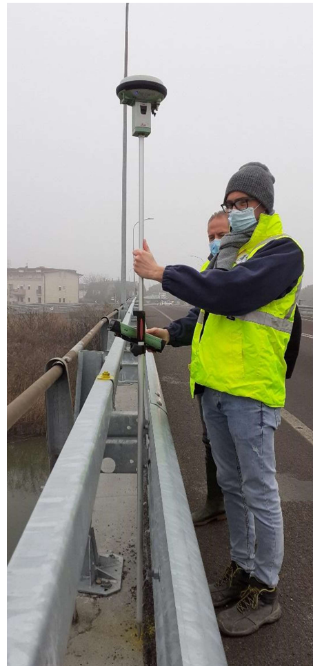
Fig. 32- maps showing the position of the monitoring point MOR_PA, measurement height and bridge height in respect of the mean sea level (on the left), topographical survey with the use of GPS antenna for the acquisition of the measured altitude (on the right)
