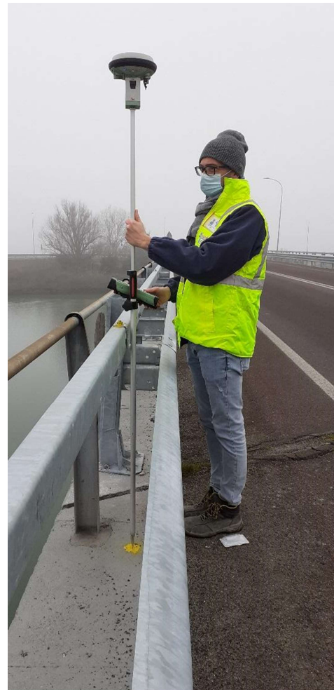
Fig. 30 – maps showing the position of the monitoring point BRE_PA, measurement height and bridge height in respect of the mean sea level (on the left), topographical survey with the use of GPS antenna for the acquisition of the measured altitude (on the right)
