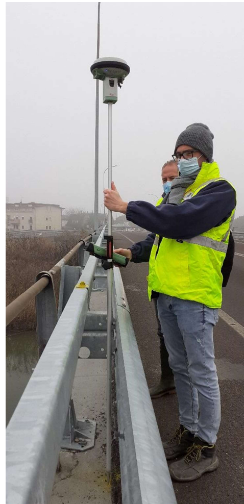
Fig. 31- maps showing the position of the monitoring point BAC_PA, measurement height and bridge height in respect of the mean sea level (on the left), topographical survey with the use of GPS antenna for the acquisition of the measured altitude (on the right)
