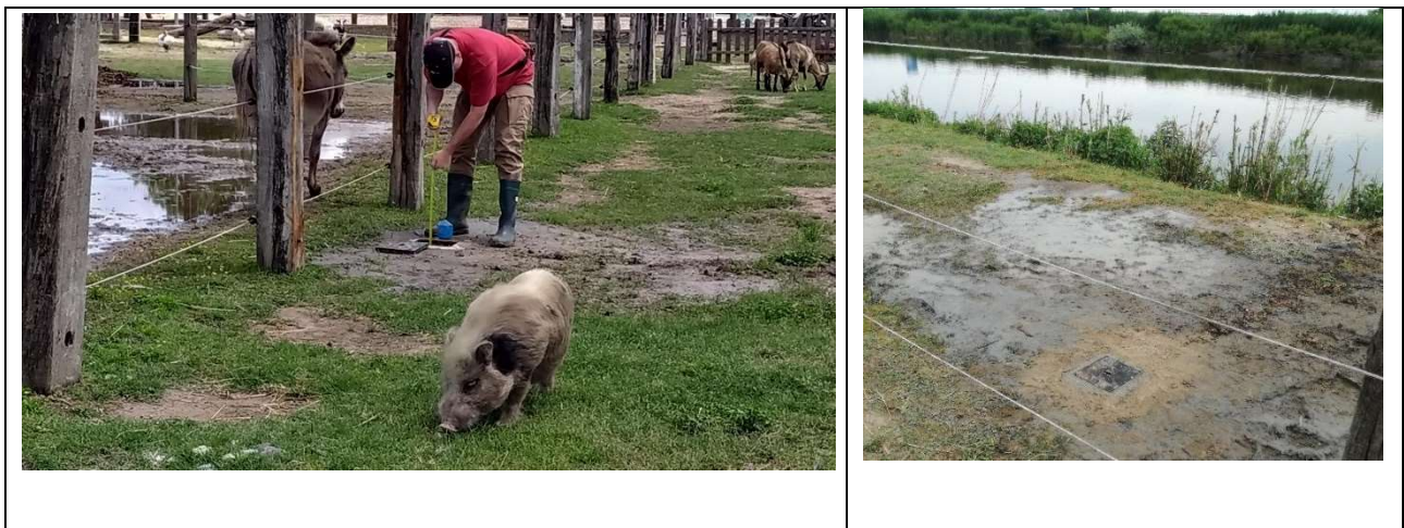
Fig. 11 – a) piezometer with underground tap and still full floor cover adopted in MoST5 to prevent damage to the animals of the farm.
