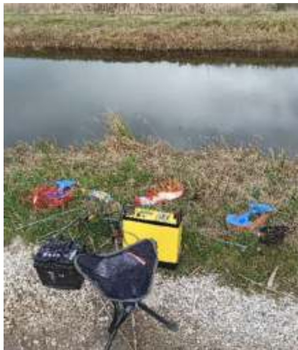
Figure 7.15 Electrical sounding on GS-100-24 position.
