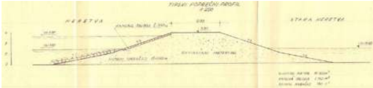
Figure 3.26 Cross section of an embankment dam at the beginning of the Stara Neretva River
