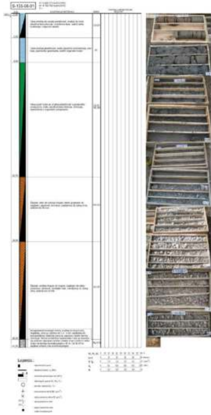
Figure 3.72 An example of borehole profile
