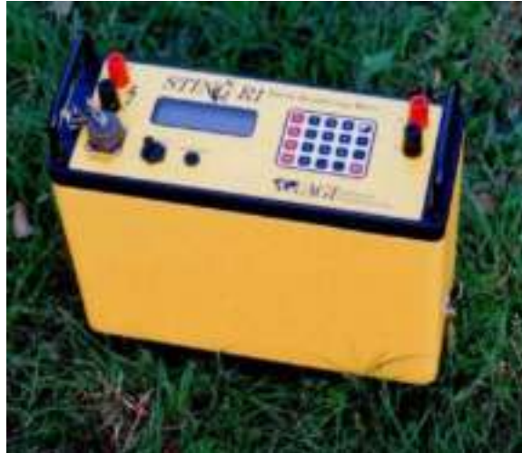
Figure 7.14 Equipment for geoelectrical sounding AGI Sting R-1
