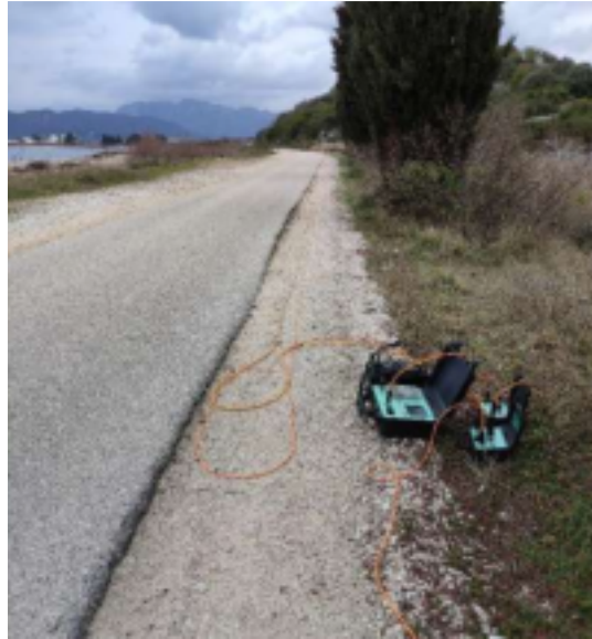
Figure 7.13 Geoelectrical tomography on GE-5 profile position.
