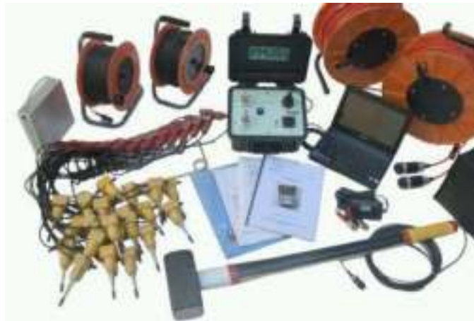
Figure 7.10 Equipment for seismic surveys.
