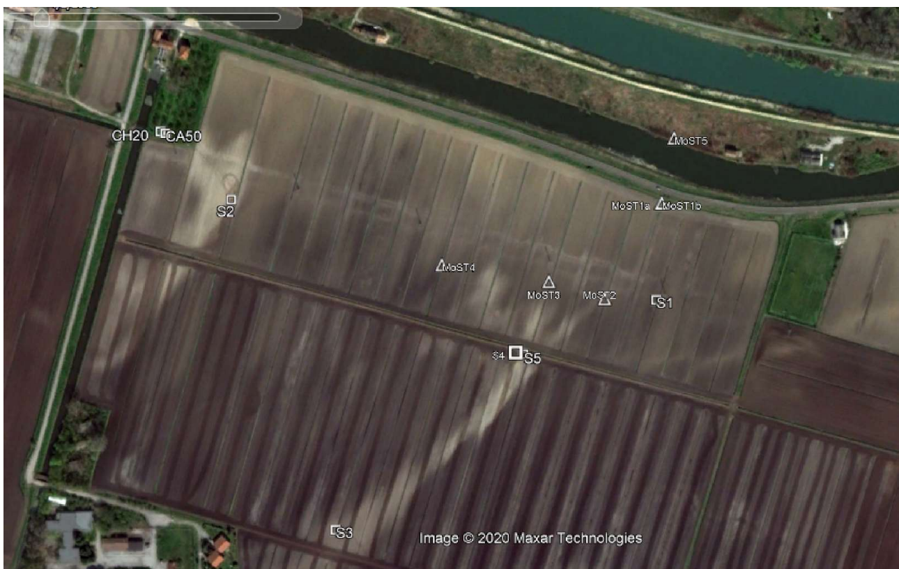
Fig. 20 - Groundwater monitoring network available for the measurements carried out in February and May 2020. The interval depth from ground surface refers to the pipe screen.
