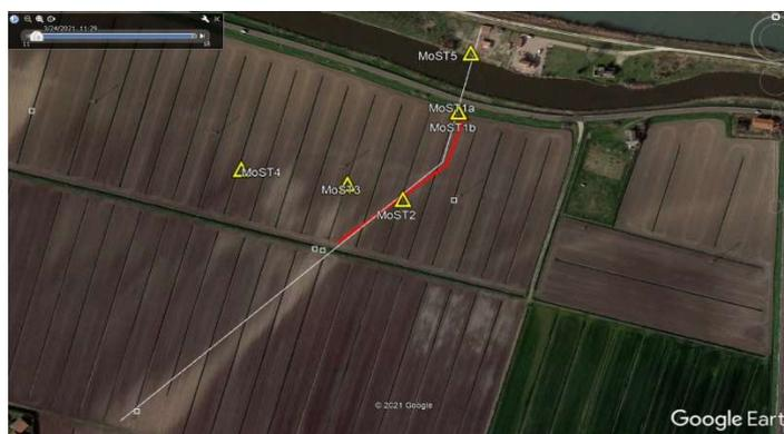
Fig. 16 – Location of the analyzed sedimentary cores (white square: S1-S5; yellow triangles MoST1-MoST5). The red and white lines represent the sub-irrigation pipe and the stratigraphic section showed in Fig. 17.
