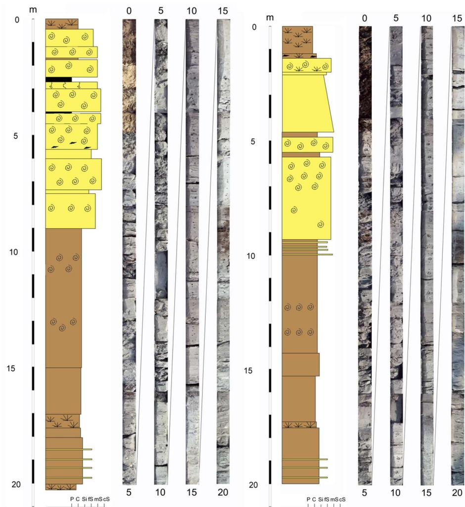
Fig. 15 - Litho-stratigraphic log of S3 and S1 sediment cores drilled in the study area.
