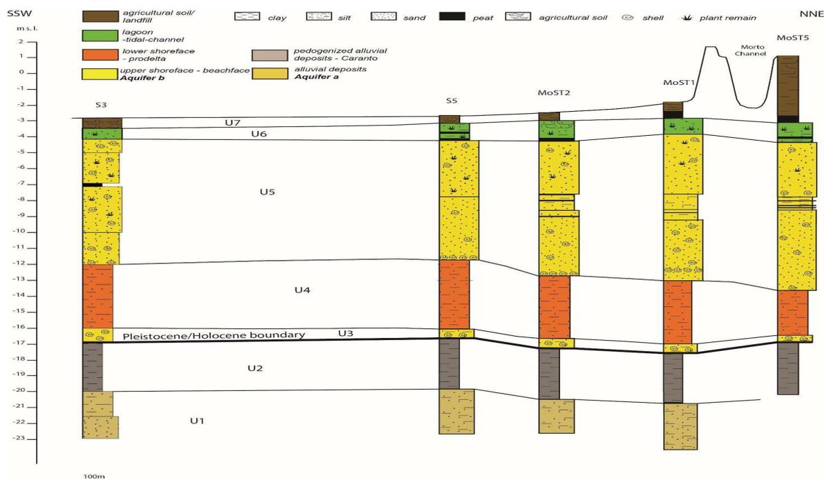
*Fig. 17 – Stratigraphic section of the pilot test site, along the surficial sandy paleo-channel (the locations of the section, of the pipe and of the analyzed cores are shown in Fig. 15).*
