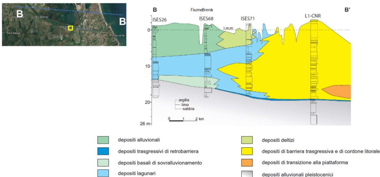
Fig. 2 – Setting of the Holocene depositional units.
