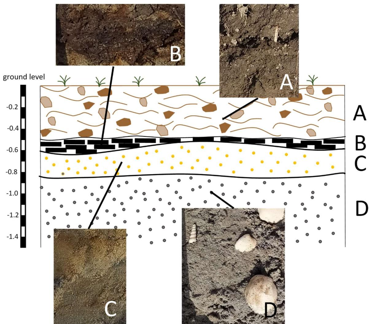
*Fig. 12 – Sketch of subsoil of the first 1.5 meters.*
