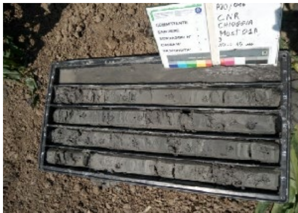
Fig. 4 - MoST1a sediment line cores 0-5m.
