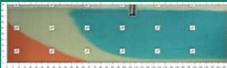
FIGURE 15. LABORATORY EXPERIMENT RESULT OF ACTIVE SEA WATER INTRUSION WITH RECHARGE CHANNEL IMPLEMENTED
