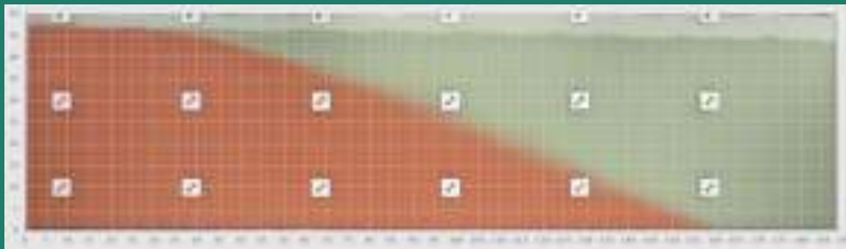
FIGURE 13. LABORATORY EXPERIMENT RESULT OF ACTIVE SEA WATER INTRUSION IN PRESENT STATE
