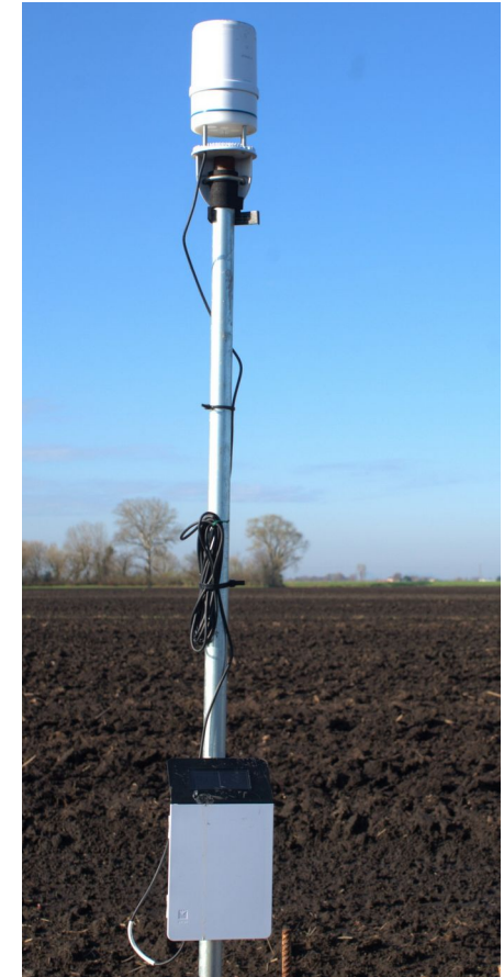
ATMOS41 all-in-one weather station with ZL6 datalogger (METER Group)
