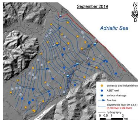
The risk related to salt intrusion in coastal aquifer has been computed with a numerical model, both at the regional and local scale, for different future scenarios (with and without well pumping). In the case of Fano, higher risk classes are related to overexploitation by irrigation, industrial (and domestic) wells; with a general lack of control of the effective pumping rate by private users and without a piezometric network able to detect their depression cones.
