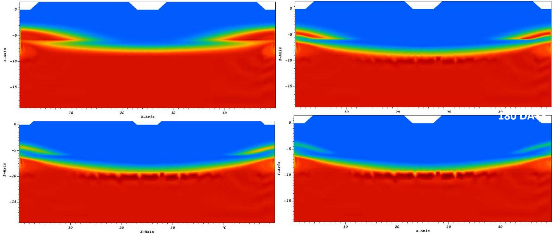
Figure 24 – Model B: solute concentration on a vertical section through the barycenter of the model after 3, 6, 9 and 12 months of aquifer recharge with  $h = 30$  cm and constant recharge during the simulation time.
