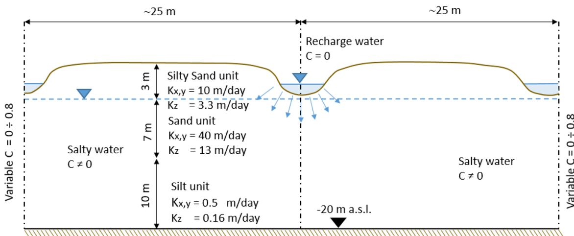
Figure 12 – Model B: Conceptual model of ditch recharge.
