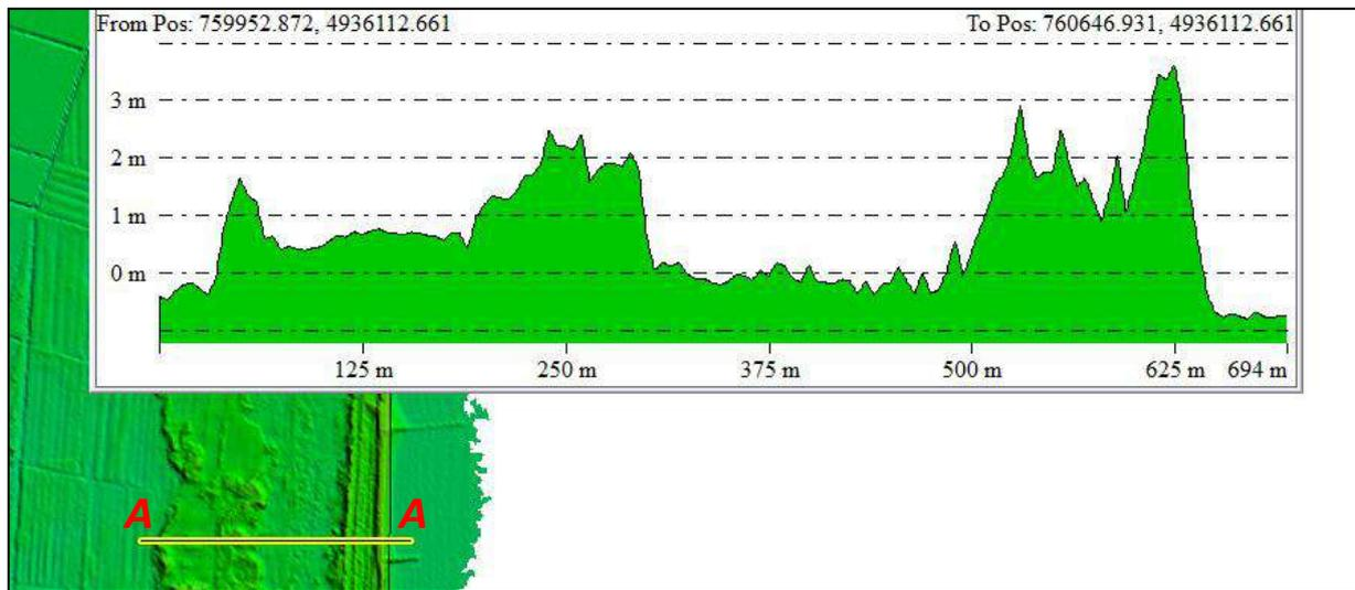
Figure 8 – Representative section profile A-A of dunes and retro dunes area extract from DEM
