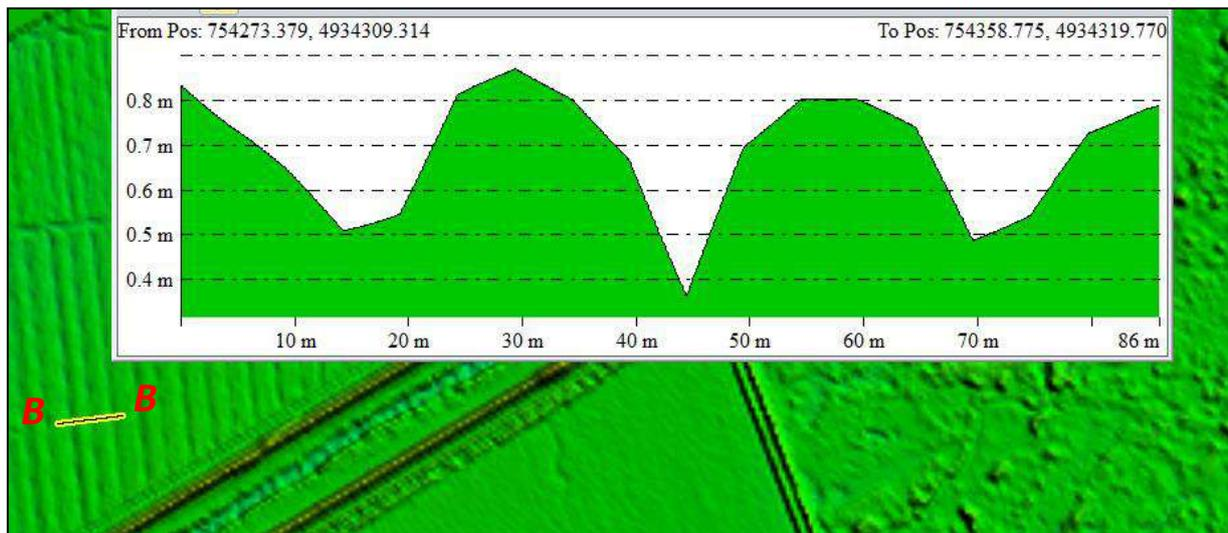
Figure 9 – Representative section profile B-B of agricultural ditches extract from DEM.
