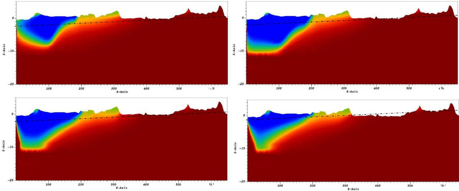
Figure 19 – Model A: solute concentration on a vertical section through the barycenter of the model after 1, 3, 4 and 6 months of aquifer recharge with  $h = 30$  cm and sea level 0.7 m asl.
