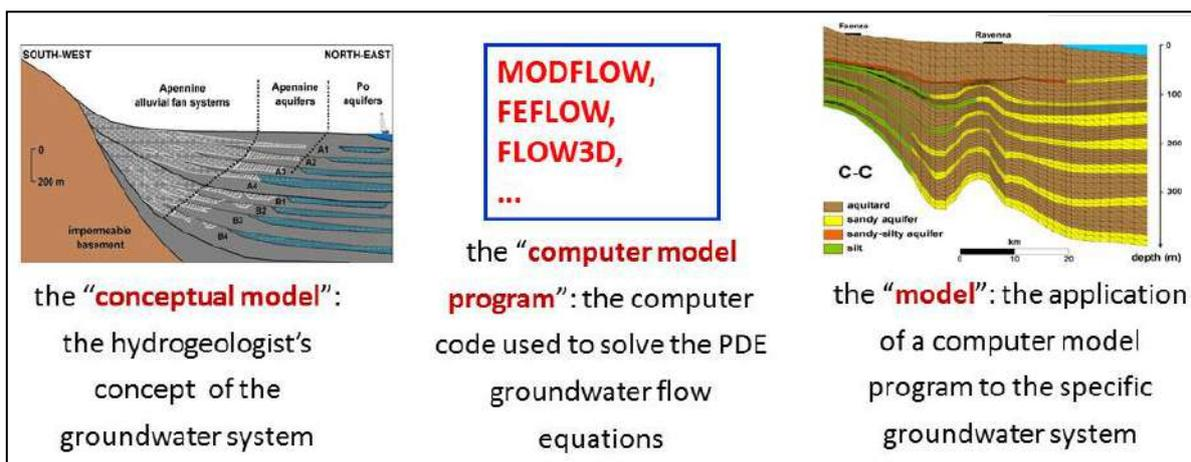
Figure 7 – Sketches representing the three model types that must be developed to simulate and manage groundwater resources and MAR
