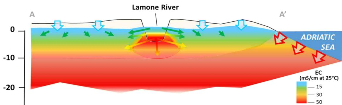
Figure 3 – Schematic conceptual model of the shallow coastal aquifer of Ravenna: 1) local rainfall infiltration; 2) seawater intrusion from the shoreline; 3) freshwater flow in superficial watercourses; 4) seawater intrusion along river beds; 5) transfer of freshwater from superficial watercourses to groundwater; 6) transfer of saline and brackish water from the superficial watercourses to groundwater; 7) trace of the section A-A'. EC= Electrical conductivity
