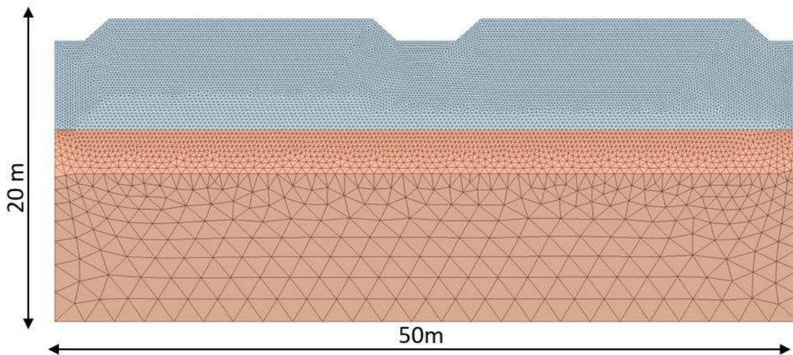
Figure 14 – Slice in the middle of three-dimensional finite element mesh of ditch recharge model (Model B).
