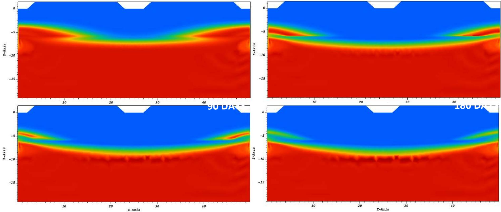
Figure 22 – Model B: solute concentration on a vertical section through the barycenter of the model after 3, 6, 9 and 12 months of aquifer recharge with  $h = 15$  cm and constant recharge during the simulation time.
