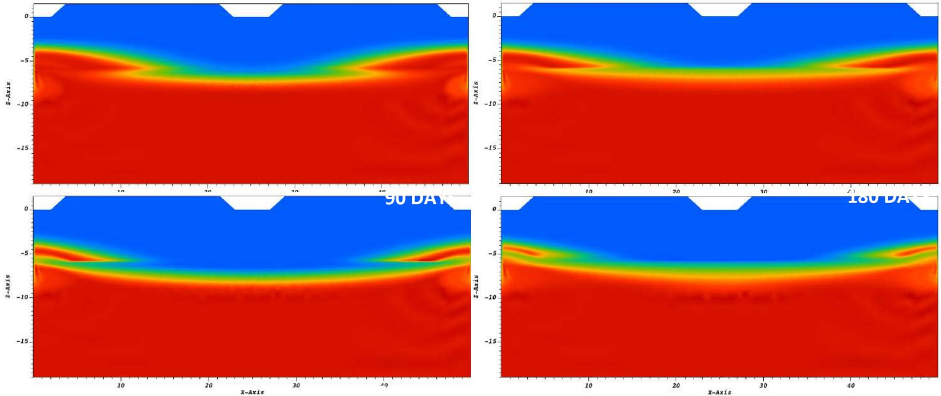
Figure 23 – Model B: solute concentration on a vertical section through the barycenter of the model after 3, 6, 9 and 12 months of aquifer recharge with  $h = 15$  cm and seasonal recharge during the simulation time.
