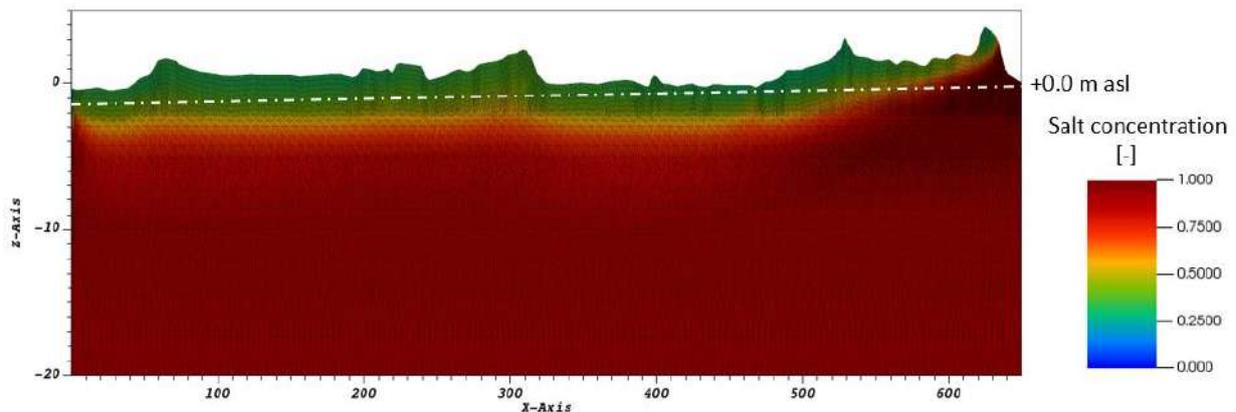
Figure 17 – Steady-State condition of model A, reached after 1 year of simulation. The white line indicates the water table imposed.
