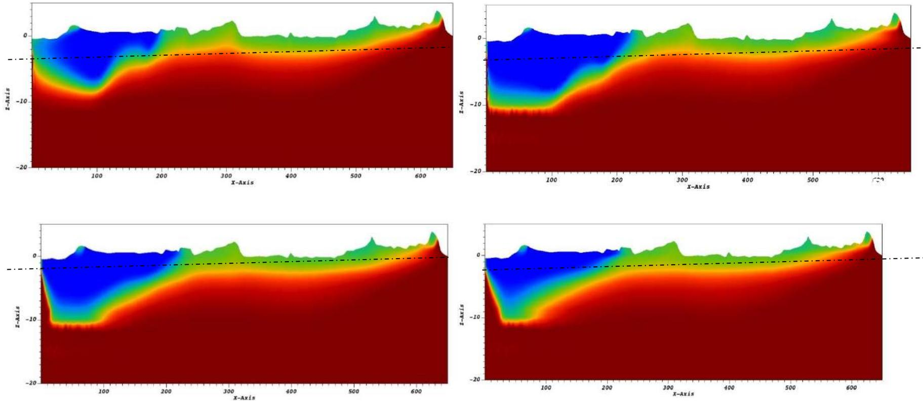
Figure 18 – Model A: solute concentration on a vertical section through the barycenter of the model after 1, 3, 4 and 6 months of aquifer recharge with  $h = 30$  cm and sea level 0.0 m asl.
