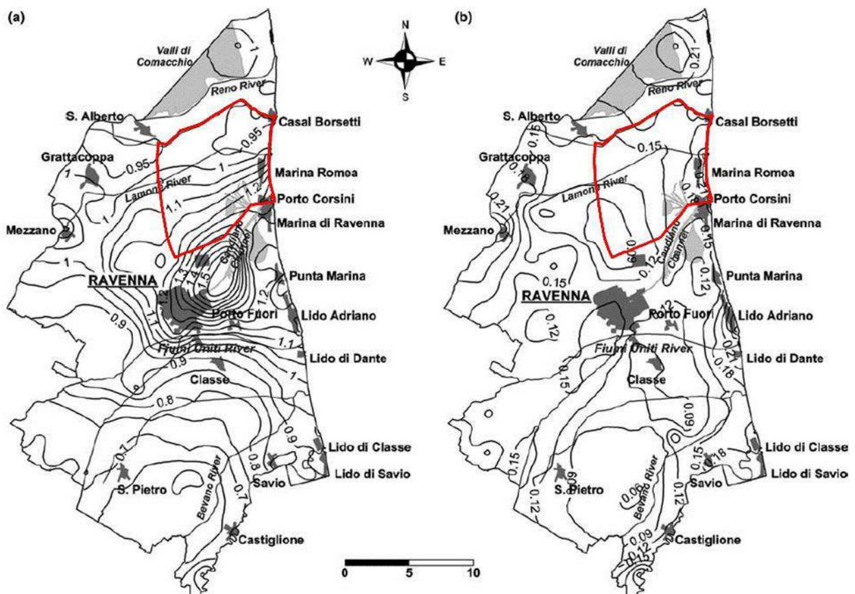
Figure 4 – Cumulative land subsidence (m) in the Ravenna Municipality a from 1897 to 2002 and b from 1977 to 2002 obtained from the GIS processing of the available leveling data. The contouring intervals are 0.05 m and 0.03 m, respectively (modified after Teatini et al., 2005). The study area is represented by a red line perimeter.
