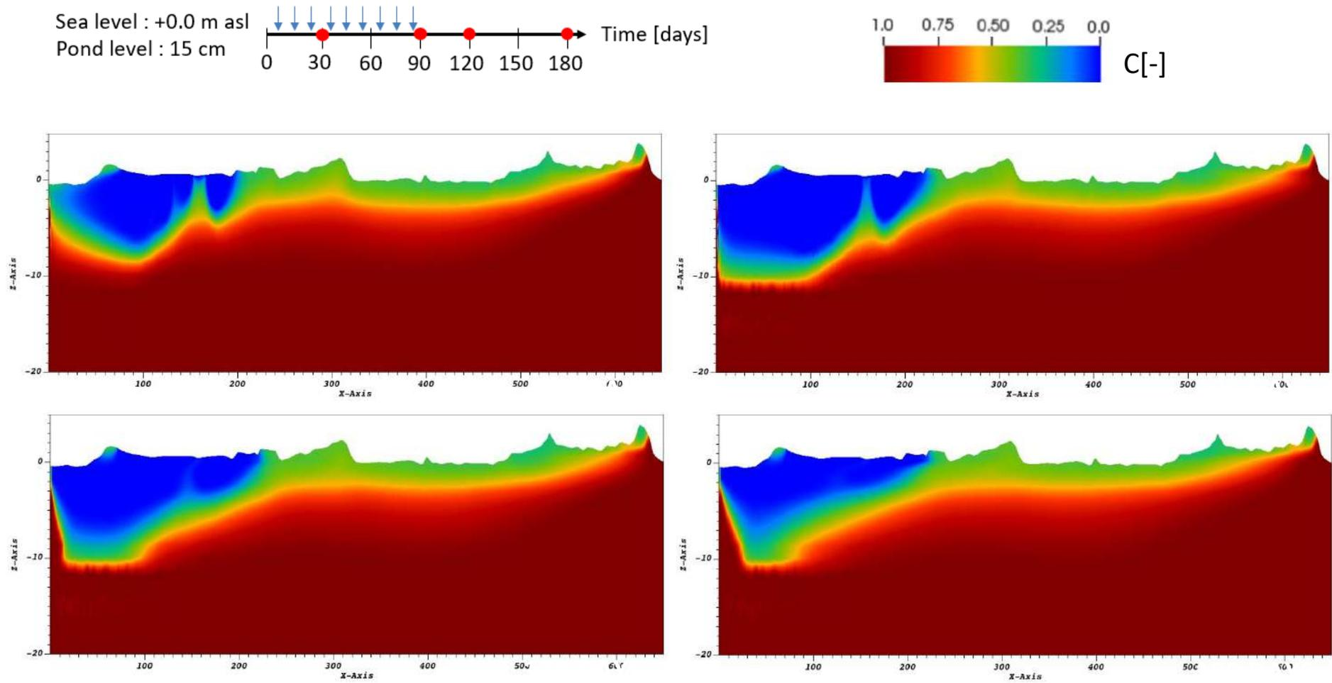
Figure 20 – Model A: solute concentration on a vertical section through the barycenter of the model after 1, 3, 4 and 6 months of aquifer recharge with  $h = 15$  cm and sea level 0.0 m asl.
