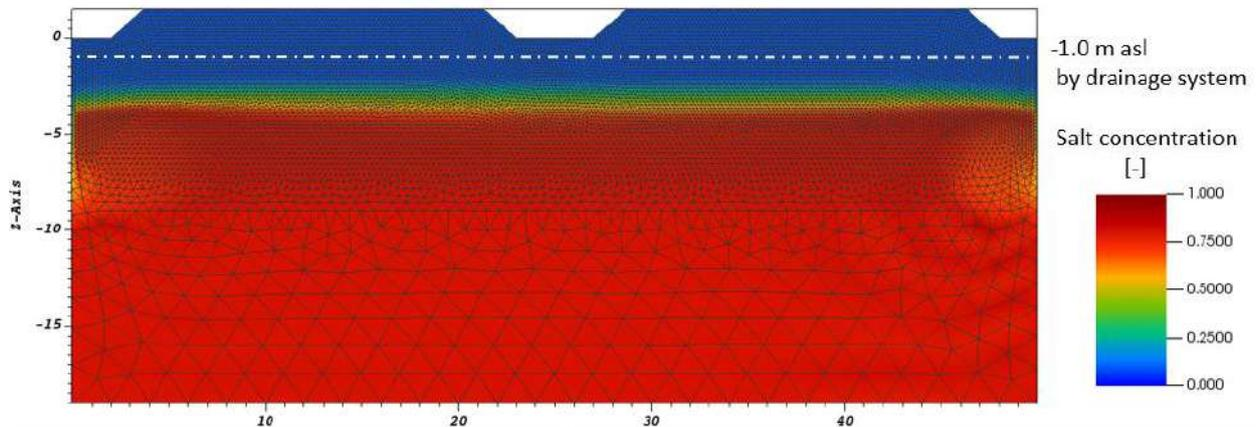
Figure 18 – Steady-State condition of model B, reached after 1 year of simulation. The white line indicates the water table imposed.
