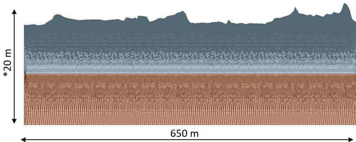
Figure 13 –Slice in the middle of three-dimensional finite element mesh of retrodune recharge model (Model A). The vertical exaggeration is 10.
