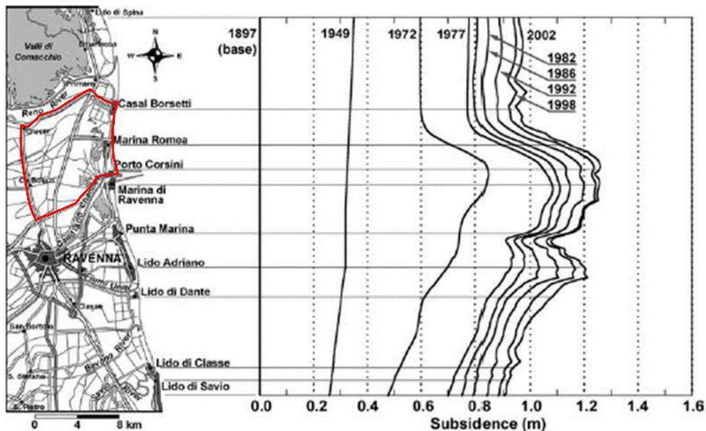
Figure 5 – Land subsidence versus time along the shoreline of the Ravenna Municipality obtained from the GIS slicing of the leveling data (modified after Teatini et al., 2005). The study area is represented by a red line perimeter.
