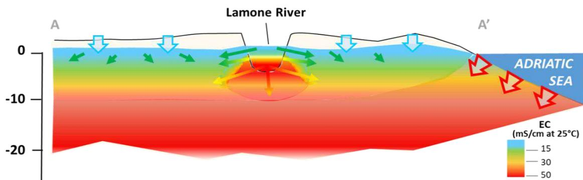
Figure 3 – Schematic conceptual model of the shallow coastal aquifer of Ravenna: 1) local rainfall infiltration; 2) seawater intrusion from the shoreline; 3) freshwater flow in superficial watercourses; 4) seawater intrusion along river beds; 5) transfer of freshwater from superficial watercourses to groundwater; 6) transfer of saline and brackish water from the superficial watercourses to groundwater; 7) trace of the section A-A'. EC= Electrical conductivity
