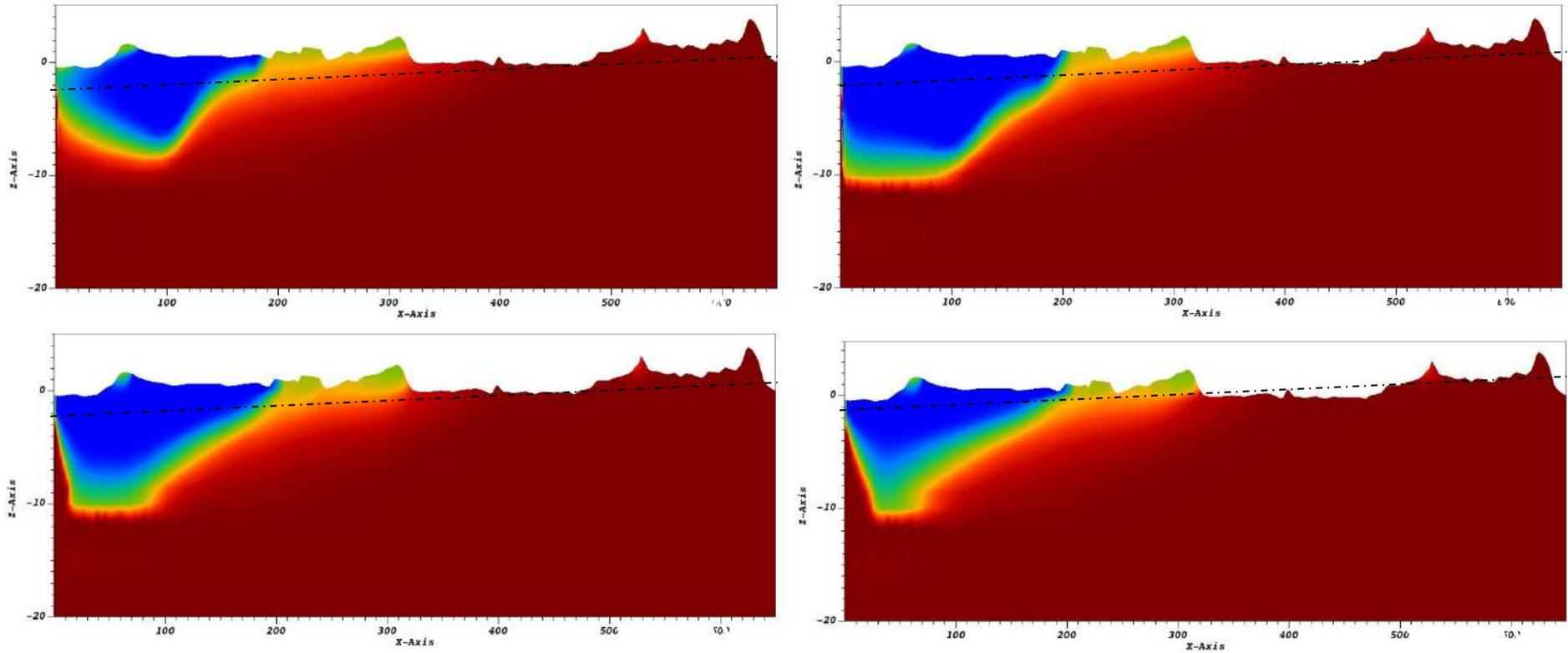
Figure 19 – Model A: solute concentration on a vertical section through the barycenter of the model after 1, 3, 4 and 6 months of aquifer recharge with  $h = 30$  cm and sea level 0.7 m asl.
