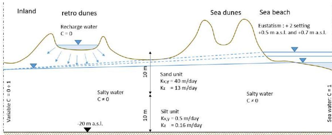
Figure 11 – Model A: Conceptual model of retrodune recharge.
