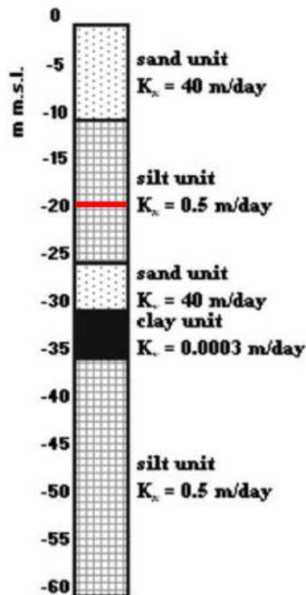
Figure 16 – Simplified subdivision of the permeable aquifer and hydraulic conductivity values ( $K_x$ ), as used in the numerical model (after Gimbastiani et al. 2007). The red line indicates the bottom layer of the developed model.
