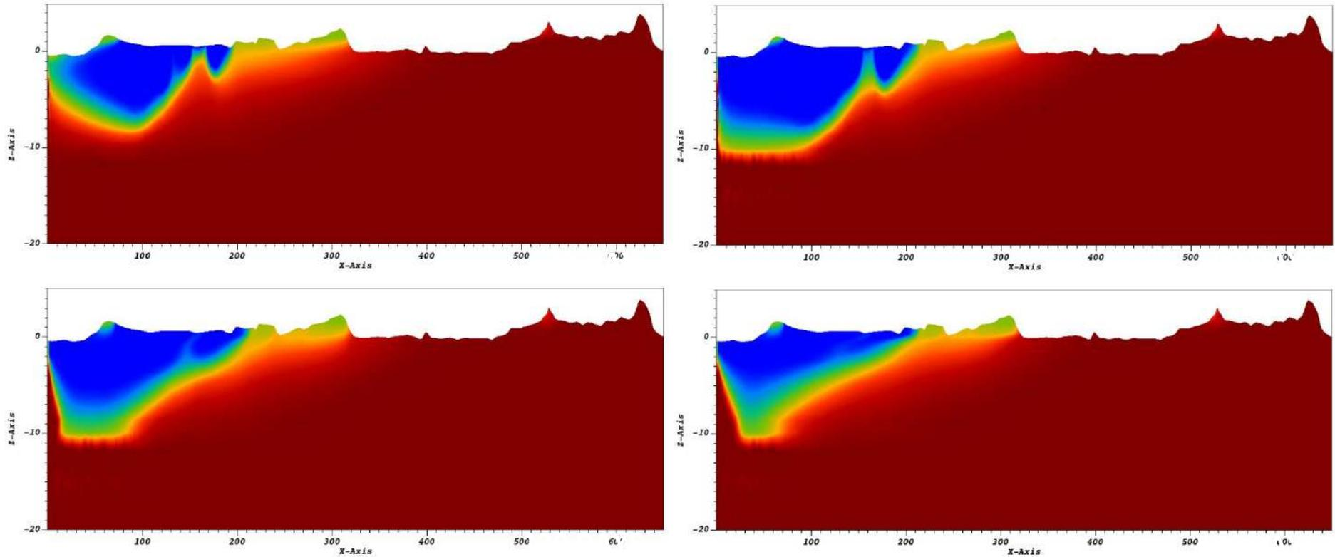
Figure 21 – Model A: solute concentration on a vertical section through the barycenter of the model after 1, 3, 4 and 6 months of aquifer recharge with  $h = 15$  cm and sea level 0.0 m asl.
