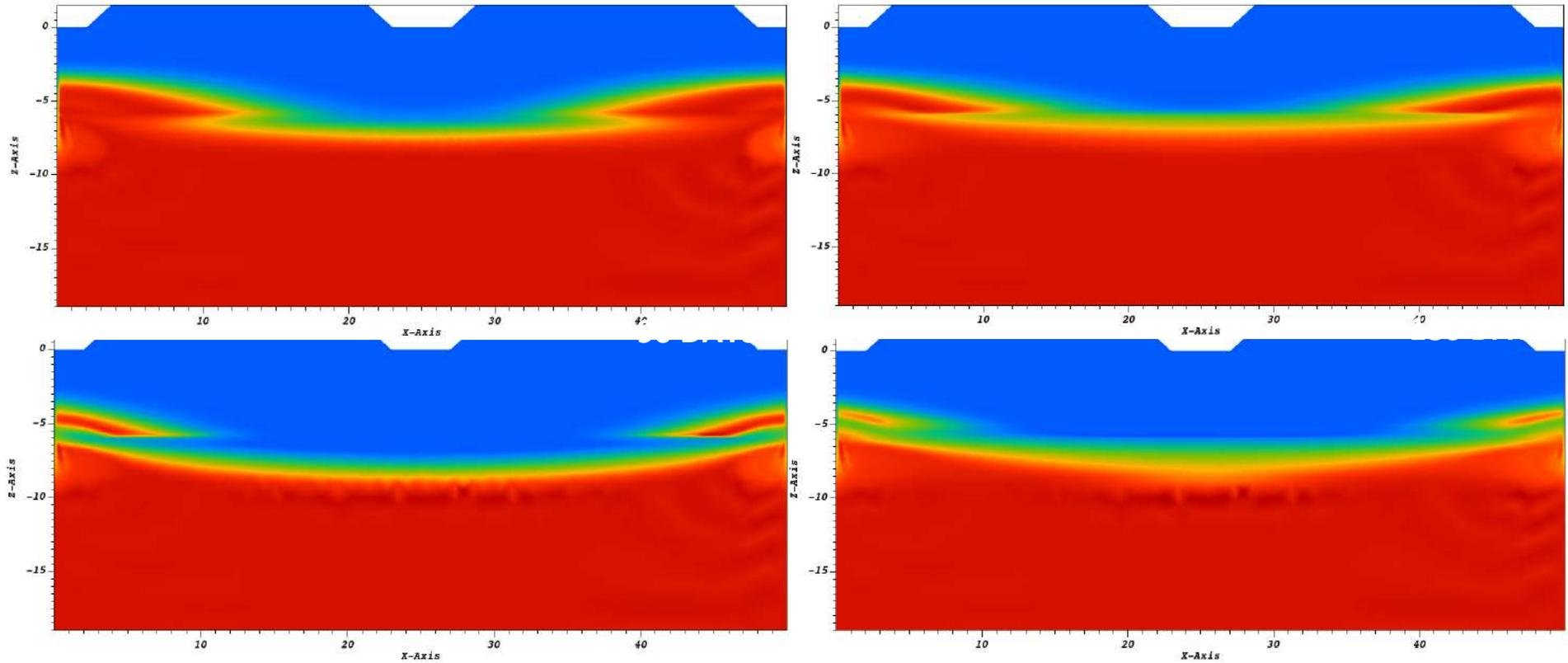
Figure 25 – Model B: solute concentration on a vertical section through the barycenter of the model after 3, 6, 9 and 12 months of aquifer recharge with  $h = 30$  cm and seasonal recharge during the simulation time
