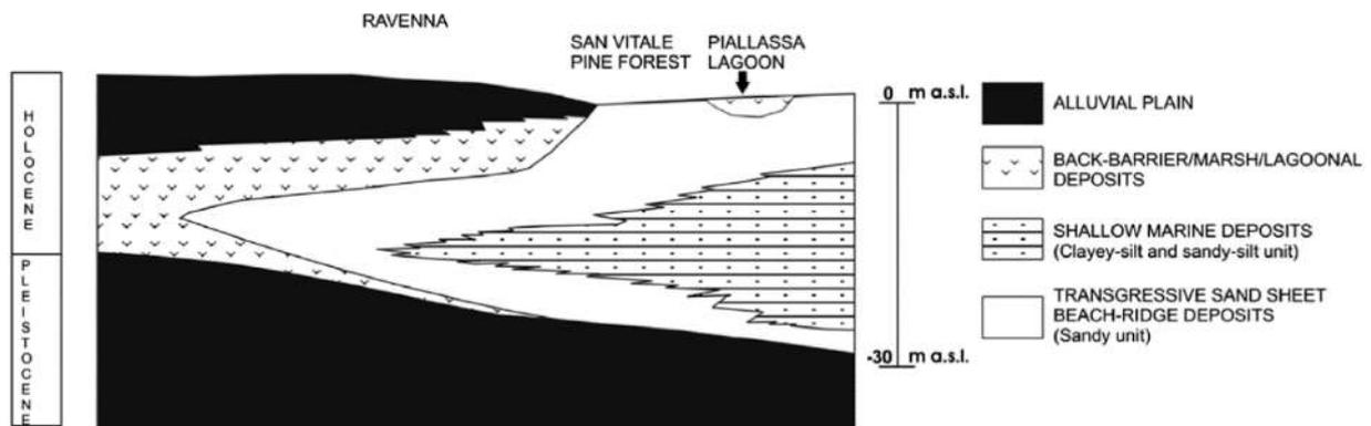
Figure 15 – Lithostratigraphic reconstruction of the study area (modified from Amorosi et al., 1999; Marchesini et al., 2000, Giambastiani et al. 2007).
