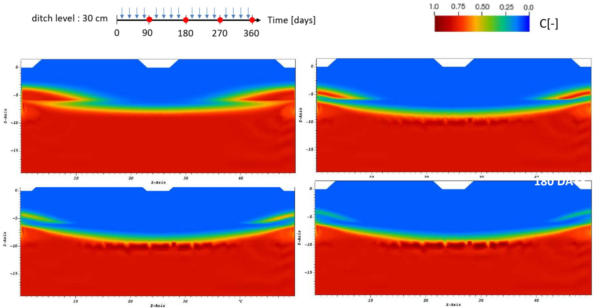
Figure 24 – Model B: solute concentration on a vertical section through the barycenter of the model after 3, 6, 9 and 12 months of aquifer recharge with  $h = 30$  cm and constant recharge during the simulation time.
