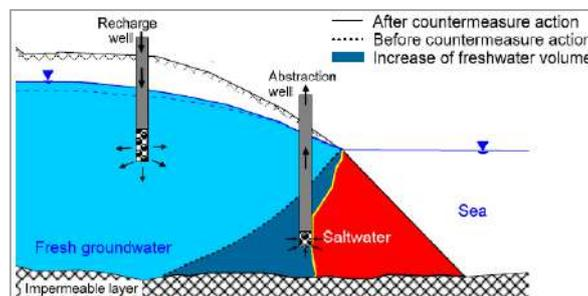
Especially in the case of confining layers, it will be possible designs systems of Cyclic Recharge with injection of freshwater during wet season followed by pumpings in the dry season. The percentage of water extracted for suitable use, referred to injected volume, defines COP of the system.
